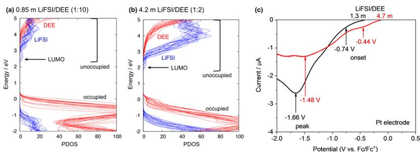
Fig. 5 Theoretical and experimental investigations on the  $\text{FSI}^-$  reduction potential. PDOS profiles of (a) dilute (0.85 m, LiFSI : DEE = 1 : 10 by mol) and (b) concentrated (4.2 m, LiFSI : DEE = 1 : 2 by mol) electrolytes. (c) LSV curves of a Pt electrode in 1.3 m and 4.7 m LiFSI/DEE at  $1 \text{ mV s}^{-1}$ . The onset and peak potentials of the reduction reactions are indicated. The onset potential was defined at the cathodic current flow of  $0.25 \mu\text{A}$ .
