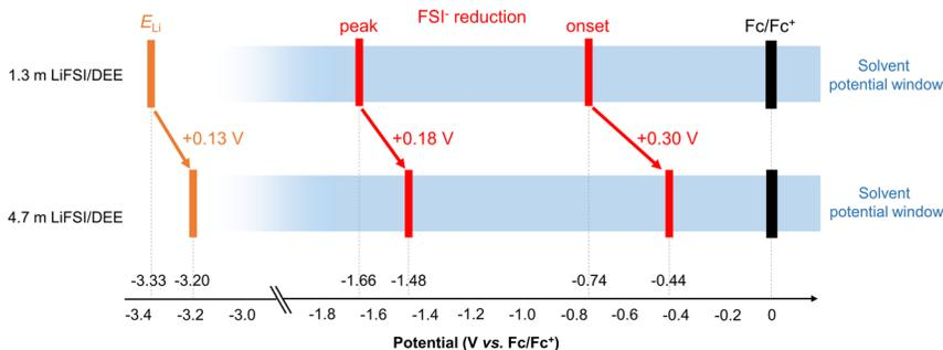
Fig. 6 Potential diagram of dilute (1.3 m) and concentrated (4.7 m) LiFSI/DEE that highlights the upward shift of  $E_{Li}$  and FSI<sup>-</sup> reduction potential.
