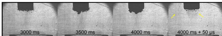
Fig. 4 Representative high-speed imaging of the cavitation development in CaDES at 25% input power over a 4 s sonication with additional representative high-speed imaging of the fully developed cavitation at 50% input power. Bubble collapse shockwaves captured by the shadowgraphic imaging are shown with yellow arrows, and scale is provided by the 6 mm- \varnothing horn tip.
