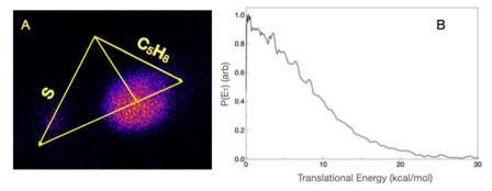
Fig. 7 (A) Sliced velocity map image of the 85 u product,  $C_4H_5S$ , for the reaction of  $S(^3P)$  with isoprene (Newton diagram superimposed) under a collision energy of 11.7 kcal mol<sup>-1</sup>. (B) Total translational energy release ( $P(E_T)$ ) extracted from image (A).
