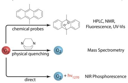
Fig. 6 Methods to detect singlet oxygen ( $^{1}O_{2}$ ) in non-aqueous oxygen redox systems. The use of 9,10-dimethylanthracene (DMA) as a chemical probe is highlighted. Figure taken from https://doi.org/10.1039/D3FD00088E.
