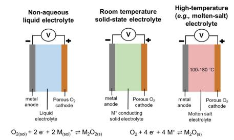
Fig. 2 Various configurations of (open) alkali-metal-O<sub>2</sub> cell chemistries.
