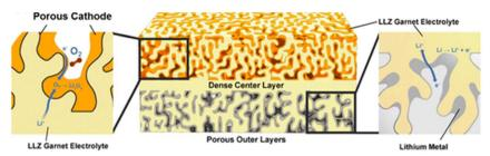
Fig. 4 Concept of a tri-layer garnet  $\text{Li}_7\text{La}_3\text{Zr}_2\text{O}_{12}$  (LLZ)  $\text{Li}-\text{O}_2$  cell with high interfacial surface area, short lithium-ion conduction pathways and minimized use of electrolyte material, taken from https://doi.org/10.1039/D3FD00119A.
