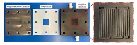
Fig. 8 Photographs of the cell housing used in the study, with a magnified image of the flow field plate shown, as taken from https://doi.org/10.1039/D3FD00137G.
