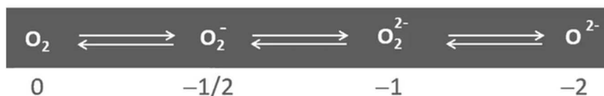
Fig. 1 Oxygen redox chemistry showing transition via addition of electrons from dioxygen gas (O 2 ) to superoxide (O 2 − ) to peroxide (O 2 2− ) to oxide (O 2− ), with the formal oxidation number written below.
