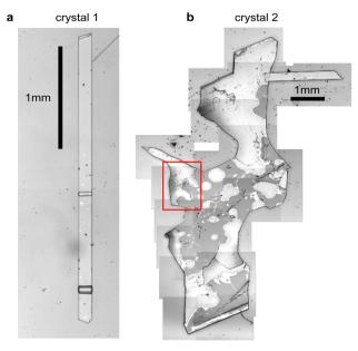
Fig. 2 Rubrene single crystals. (a and b) Microscope images of crystals 1 and 2, respectively, grown by physical vapour transport. All spectroscopic measurements of crystal 2 were conducted within the region indicated by the red box.
