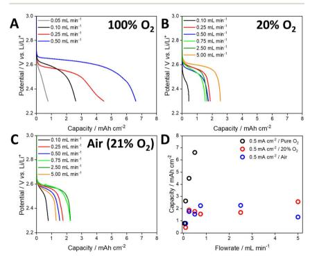
Fig. 3 Discharge profiles of cells discharged at a current density of 0.5 mA cm $^{-2}$  under a flow of (A) 100%  $O_2$ , (B) 20%  $O_2$  with  $N_2$  balance and (C) air. (D) Shows the areal capacity of these cells.
