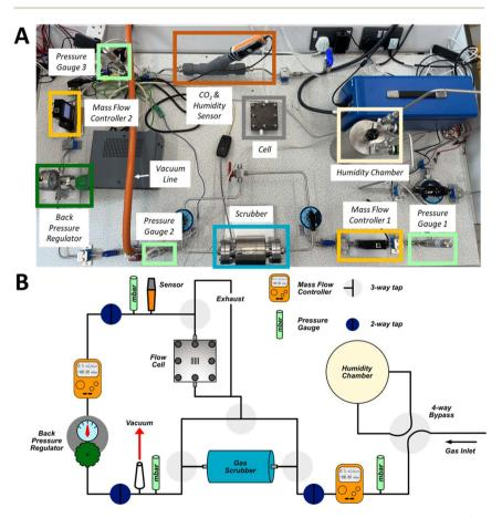
Fig. 1 (A) Photograph of the Li–air demonstrator system with labelled components. (B) A schematic diagram of the Li–air demonstrator system. A description of the design can be found in the text.
