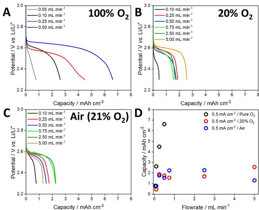
Fig. 3 Discharge profiles of cells discharged at a current density of 0.5 mA cm<sup>-2</sup> under a flow of (A) 100% O<sub>2</sub>, (B) 20% O<sub>2</sub> with N<sub>2</sub> balance and (C) air. (D) Shows the areal capacity of these cells.
