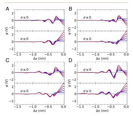
Fig. 5 Interface electric potential as a function of distance from the electrode,  $\Delta x$ . Colours blue  $\rightarrow$  red indicate increasing solution charge densities from  $|\sigma|=0 \rightarrow 0.77e~\text{nm}^{-2}$ . (A)–(D) are taken from simulations where the target bulk ion concentration was 0, 1, 5 and 10 M, respectively.
