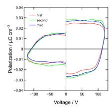
Fig. 6 P-V hysteresis curves of the MISIM ([ITO|PC|ET-PRBT|PC|Aq]) device at room temperature.
