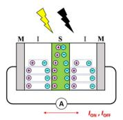
Scheme 2 Operating mechanism of the MISIM photocell. Light irradiation induces synergetic polarizations in the S and I layers, while blocking leads to their depolarization, leading to AC in the external circuit.
