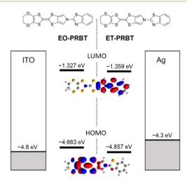
Fig. 1 Energy diagram for the HOMOs and LUMOs of ET-PRBT and EO-PRBT, and for the work functions of ITO and Ag electrodes.
