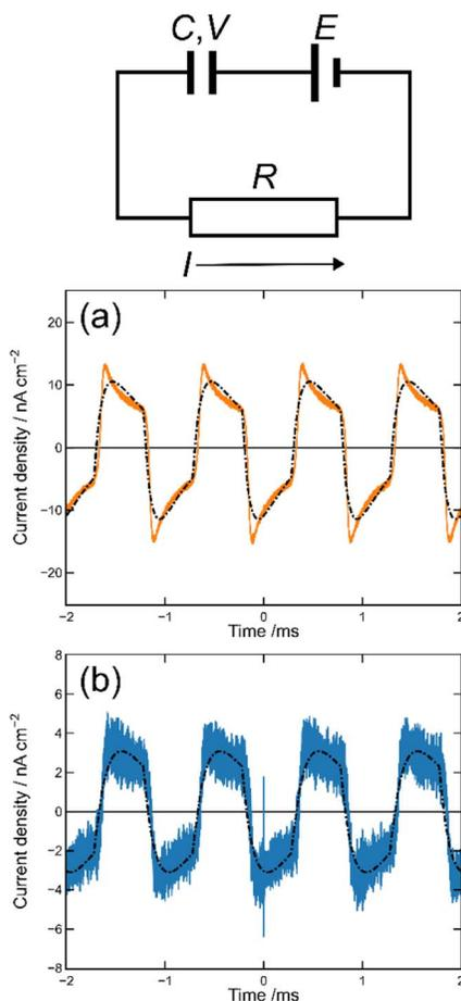
Fig. 5 Results of the photocurrent analysis in the MISIM photocells with  $S = \text{ET-PRBT}$  (a) and  $S = \text{EO-PRBT}$  (b). The broken curves represent the theoretical best fits of eqn (1) and (2). The inset schematically shows the model circuit for the MISIM photocell, where  $E$  corresponds to the voltage of the S layer,  $C$  and  $V$  to the capacitance and voltage of the I layers, respectively, and  $I$  and  $R$  to the current flowing and the effective resistance, respectively.
