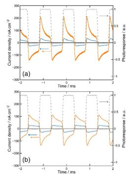
Fig. 3 Time trajectory of the transient photocurrent for the [ITO|I|S|Ag] (a) and [ITO|S|I|Ag] (b) photocells. The orange and blue curves show the photocurrents when S = ET-PRBT and EO-PRBT, respectively, and the gray broken curves indicate the response from a SI diode to monitor the light-on and -off periods.
