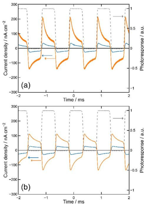
Fig. 3 Time trajectory of the transient photocurrent for the [ITO||S||Ag] (a) and [ITO||S||Ag] (b) photocells. The orange and blue curves show the photocurrents when  $S = \text{ET-PRBT}$  and  $\text{EO-PRBT}$ , respectively, and the gray broken curves indicate the response from a Si diode to monitor the light-on and -off periods.
