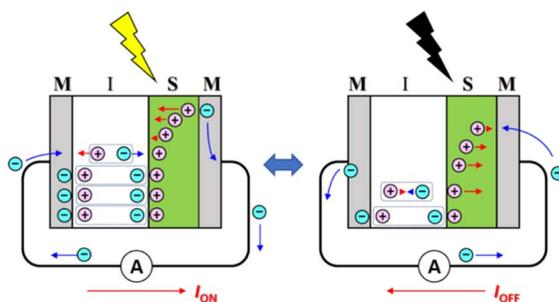
**Scheme 1** Operating mechanism of the MISM photocell. During light irradiation, charge separation occurs in the S layer, and the resulting carriers induce polarization in the I layer. This polarization synergistically enhances charge separation in the S layer, leading to a significant transient photocurrent in the external circuit ( $I_{\text{ON}}$ ). During light-off, depolarization takes place in the I layer, causing a reverse current to appear in the external circuit ( $I_{\text{OFF}}$ ).
