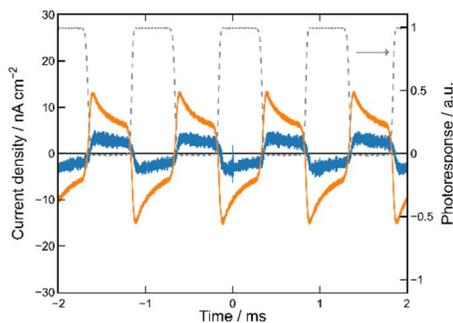
Fig. 4 Time trajectory of the transient photocurrent for the [ITO||S||Ag] photocell. The orange and blue curves show the photocurrents when  $S = \text{ET-PRBT}$  and  $\text{EO-PRBT}$ , respectively, and the gray broken curve indicates the response from a Si diode to monitor the light-on and -off periods.
