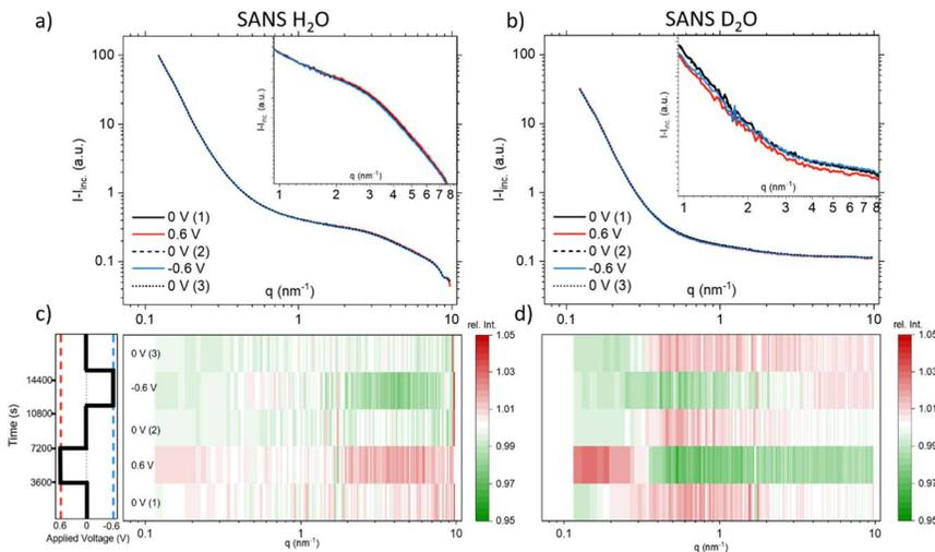
Fig. 4 Coherent SANS scattering curves and corresponding heat-plots displaying relative intensity changes for H<sub>2</sub>O (a) and (c), and D<sub>2</sub>O (b) and (d).
