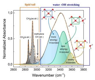
Fig. 5 Fitting example of FTIR spectra in the region  $2600-3800~{\rm cm}^{-1}$  of M70-W30 at 30 ° C. The inserted schematics represent the three different types of OH configuration in the water network.
