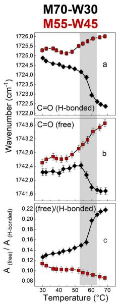
Fig. 7 Wavenumber trends of (a) hydrogen-bonded and (b) free C=O bands, and (c) intensity ratio of high (free C=O) to low (H-bonded C=O) frequency components of the carbonyl stretching band of M70-W30 (black points) and M55-W45 (red points).
