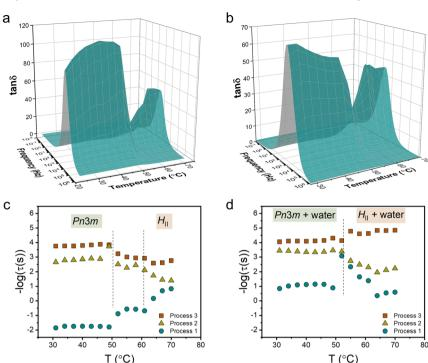
Fig. 3 3D dielectric spectra of  $\tan \delta$  as a function of frequency and temperature for (a) M70-W30 and (b) M55-W45 lipidic mesophases. Relaxation times obtained from fitting  $\tan \delta$  to the (c) M70-W30 and (d) M55-W45 lipidic mesophase. The dashed lines indicate the phase transition temperatures obtained from SAXS.
