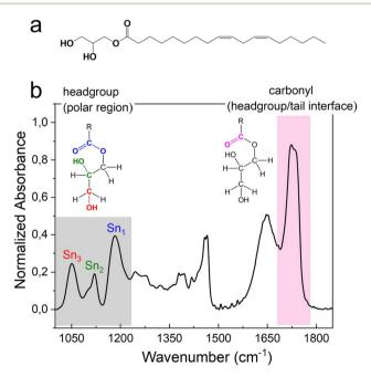
Fig. 4 (a) Molecular structure of monolinolein. (b) FTIR spectra in the region 1000–1850 cm $^{-1}$  of M70-W30 obtained at 30 °C. The Sn<sub>1</sub>, Sn<sub>2</sub>, Sn<sub>3</sub> in the grey area indicate the corresponding vibrational motions associated to the headgroup. The headgroup/tail interface, ester C=O stretching at  $\sim$ 1730 cm $^{-1}$ , is highlighted in pink.
