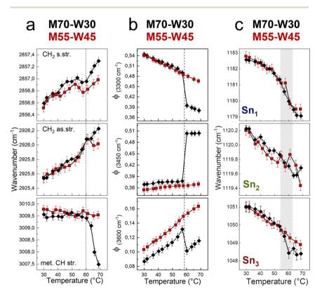
Fig. 6 (a) Wavenumber trends of the  $CH_2$  symmetric,  $CH_2$  asymmetric, and methylene CH stretching bands. (b) Fraction of strongly H-bonded, less strongly H-bonded, and weak H-bonded water molecules. (c) Wavenumber trends of  $Sn_1$ ,  $Sn_2$ , and  $Sn_3$  bands, as a function of temperature of M70-W30 (black points) and M55-W45 (red points).
