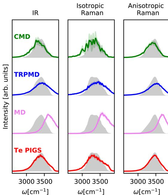
Fig. 2 IR and Raman stretching band of liquid water at 300 K with the  $T_e$  PIGS (red), MD (pink), TRPMD (blue), and CMD (green) and the experimental spectra<sup>87,88</sup> (shifted by  $22\text{ cm}^{-1}$  to account for the missing quantum coherence effects in simulation methods) in grey. All simulations are performed with a BPNN with SPC charges trained at the revPBE0-D3 level of theory.
