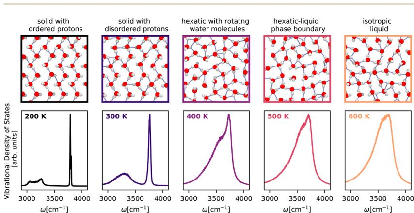
Fig. 5 Temperature-dependent vibrational density of states of monolayer water<sup>25</sup> across the solid–hexatic–liquid phase transition at a lateral pressure of 1 GPa calculated using the  $T_e$  PIGS method. The spectra are colour-coded according to temperature. The top panels (border colours indicating temperatures) correspond to snapshots of monolayer water structures. All simulations are performed with a BPNN trained at the revPBE0–D3 level of theory.
