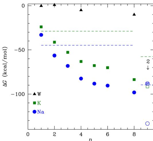
Fig. 2  $\Delta G$  as a function of the number of NMA ligands,  $n$ , for  $K^+$ ,  $Na^+$  and water (W). Horizontal dashed lines give the calculated free energy for ion hydration, which defines the reference state. The open points are for occupancy by two cations and the point with SP inside is from a single point calculation; see text for details.
