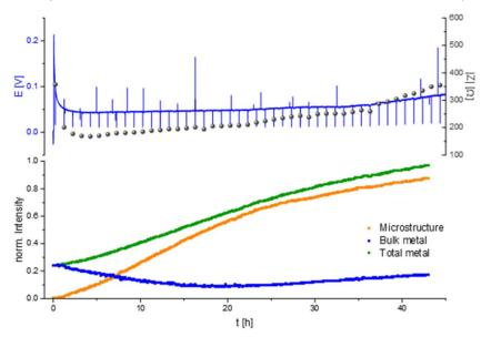
Fig. 7 Operando  $^{7}$ Li NMR and impedance (GEIS) measured at 8 Hz. Intensities measured during unidirectional Li plating at 0.5 mA cm $^{-2}$  in an NMR *in situ* cylindrical symmetrical Li cell with LP30 electrolyte.
