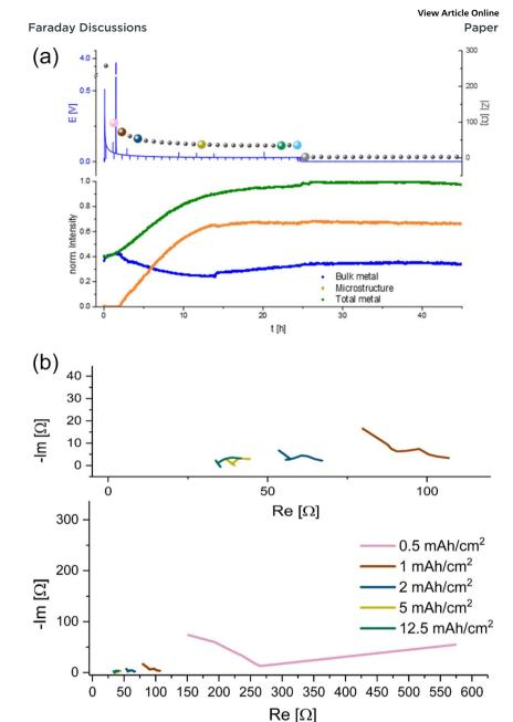
Fig. 9 (a) Operando  $^7$ Li NMR and impedance (GEIS) measured at 9 Hz. Intensities measured during unidirectional Li plating at 1 mA cm $^{-2}$  in an NMR in situ cylindrical symmetrical Li cell with LP30 + 10% FEC electrolyte. (b) GEIS Nyquist plots measured with 100  $\mu$ A amplitude during Li plating at 1 mA cm $^{-2}$  in an NMR in situ cylindrical symmetric cell, using LP30 + FEC electrolyte with GF separator at RT. Magnification of the plot at 5–15 mA h cm $^{-2}$ .
