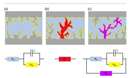
Fig. 1 Illustrations and equivalent circuits for charge transport through electrode—electrolyte interface (purely ion transport) (left; (a)), hard short circuit (electron transport) (middle; (b)), soft short circuit (mixed electron and ion transport) (right; (c)).
