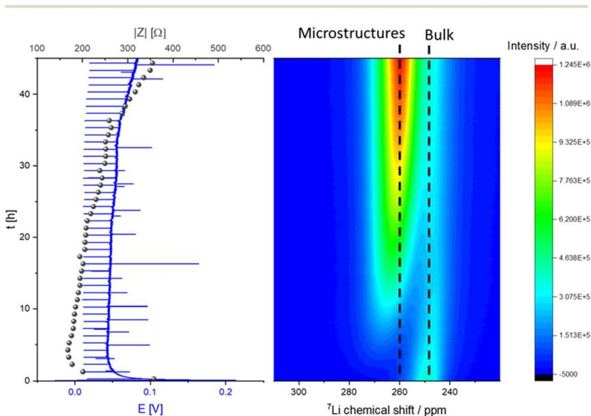
Fig. 6 *Operando* NMR spectra of unidirectional Li deposition in an NMR *in situ* cylindrical symmetrical Li cell with LP30 electrolyte (right) with corresponding voltage profile and impedance (GEIS) intensity measured at 9 Hz (left) during galvanostatic plating with a current density of  $0.5 \text{ mA cm}^{-2}$ .
