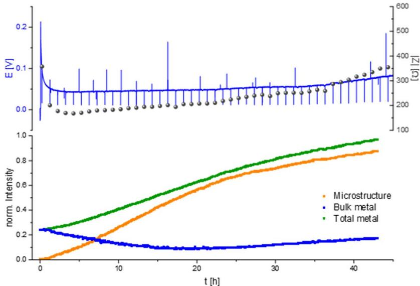
Fig. 7 *Operando*  $^7\text{Li}$  NMR and impedance (GEIS) measured at 8 Hz. Intensities measured during unidirectional Li plating at  $0.5 \text{ mA cm}^{-2}$  in an NMR *in situ* cylindrical symmetrical Li cell with LP30 electrolyte.
