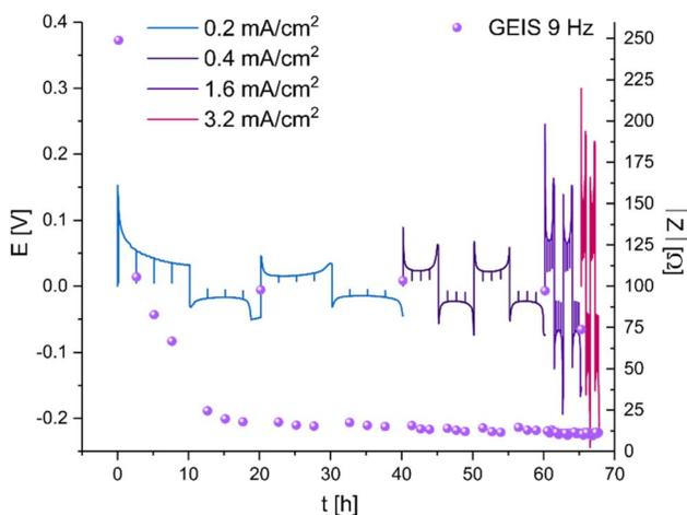
Fig. 5 Voltage traces ( $E-t$ ) of galvanostatic plating of  $1 \text{ mA h cm}^{-2}$  Li at increasing current densities between  $0.2$  and  $3.2 \text{ mA cm}^{-2}$  in a Li symmetric cell, LP30 electrolyte and GF separator at RT. EIS intensity (purple spheres) measured with GEIS at  $9 \text{ Hz}$  with  $100 \mu\text{A}$  amplitude.
