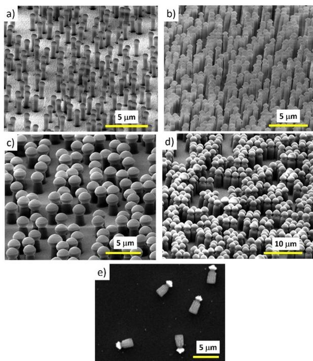
Fig. 5 Scanning electron microscope images of different Nafion arrays generated by colloidal lithography with the RIE technique. In (a) and (b) microparticles with diameters of 1  $\mu\text{m}$  have been used as masks and 0.1 and 0.2% of particle dispersions, respectively. In (c) and (d) 2  $\mu\text{m}$  diameter microparticles have been used as masks and 0.2% of particle dispersions but different RIE times (3 and 4 minutes, respectively). (e) Dispersed particles after an ultrasonic bath.
