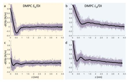
Fig. 5 3D AFM force gradient vs. tip-sample distance profiles obtained at the interface of a DMPC SLB in its  $S_o$  phase (a, c) and  $L_d$  phase (b, d). During 3D AFM imaging, some panels did not show any oscillatory hydration structures but only the monotonic contribution to the force (a, b), whilst in others the presence of hydration layers was evident (c, d). The average curve is plotted as a black thick line.
