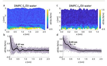
Fig. 4 Force gradient xz panels obtained at the interface of DMPC SLBs in the  $S_{\rm o}$  phase (a) and  $L_{\rm d}$  phase (c) in DI water. The corresponding force vs. tip-sample distance profiles are shown in (b) and (d), respectively. The average curve is plotted as a black thick line. Both interfaces are characterised by two hydration layers within the first nm from the lipid surface.
