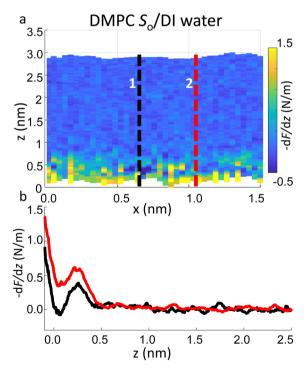
Fig. 6 (a) 3D AFM force gradient xz panel showing lateral resolution of the interfacial hydration at the surface of  $S_o$  lipids. Force gradient vs. tip-sample distance profiles obtained at position 1 and 2 in (a) are plotted in (b). Whilst in profile 2 (red curve) a hydration layer and monotonic repulsion are both evident, only the latter contribution disappears in profile 1 (black curve).
