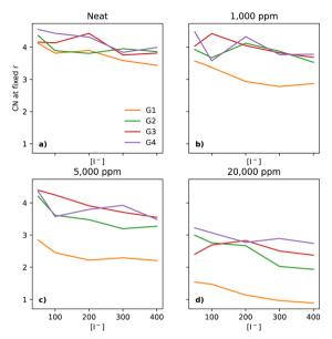
Fig. 7 Coordination number of  $I^-$  to O (of the glymes) at a fixed distance of 5 Å, for the four different glymes (G1 = yellow, G2 = green, G3 = red, G4 = purple) studied here, across the four different water concentrations (from left to right: (a) dry, (b) 1k, (c) 5k, and (d) 20k ppm of water).
