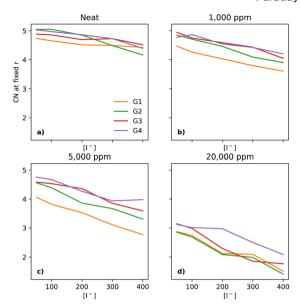
Fig. 8 Coordination number of Li $^+$  to O (of the glymes) at a fixed distance of 3 Å, for the four different glymes (G1 = yellow, G2 = green, G3 = red, G4 = purple) studied here, across the four different water concentrations (from left to right: (a) dry, (b) 1k, (c) 5k, and (d) 20k ppm of water).
