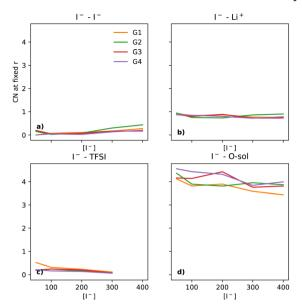
Fig. 3 The CNs of I<sup>-</sup> to (a) I<sup>-</sup>, (b) Li<sup>+</sup>, (c) TFSI and (d) O (of the solvent) captured at fixed points. The fixed points chosen were 5 Å, 3 Å, 4.5 Å and 5 Å for I<sup>-</sup>, Li<sup>+</sup>, TFSI and O (of solvent), respectively.
