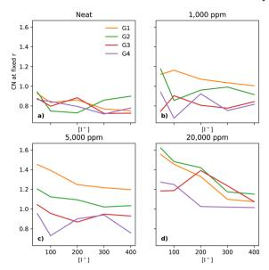
Fig. 5 Coordination number of  $I^-$  to  $Li^+$  at a fixed distance of 3 Å, for the four different glymes (G1 = yellow, G2 = green, G3 = red, G4 = purple) studied here, across the four different water concentrations (from left to right: (a) dry, (b) 1k, (c) 5k, and (d) 20k ppm of water).
