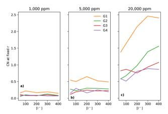
Fig. 6 Coordination number of I $^-$  to H (of H $_2$ O) at a fixed distance of 3 Å, for the four different glymes (G1 = yellow, G2 = green, G3 = red, G4 = purple) studied here, across the three water concentrations where water is present (from left to right: (a) 1k, (b) 5k and (c) 20k ppm of water).
