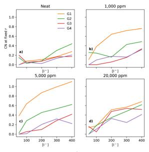
Fig. 4 CNs of  $I^-$  to  $I^-$  at a fixed distance of 5 Å, for the four different glymes (G1 = yellow, G2 = green, G3 = red, G4 = purple) studied here, across the four different water concentrations (from left to right: (a) dry, (b) 1k, (c) 5k, and (d) 20k ppm of water). Note that (a) is a subset of the data shown in Fig. 3.
