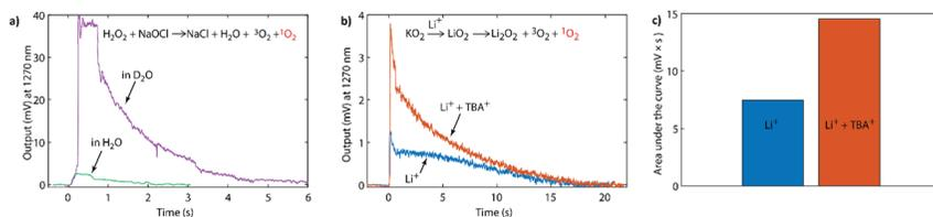
Fig. 2 (a) NIR-PMT signal upon injecting 0.5 mM NaOCl in water into 0.5 mM H<sub>2</sub>O<sub>2</sub> with the solvent being either H<sub>2</sub>O or D<sub>2</sub>O. (b) NIR-PMT signal upon injecting 100 mM LiTFSI in CH<sub>3</sub>CN, or 100 mM Li<sup>+</sup> : TBA<sup>+</sup> (1 : 9) TFSI<sup>-</sup> in CH<sub>3</sub>CN, into 1 mL suspension of KO<sub>2</sub> mixed with 50 mM 18-crown-6 in CH<sub>3</sub>CN. (c) The integrated signals from (b).
