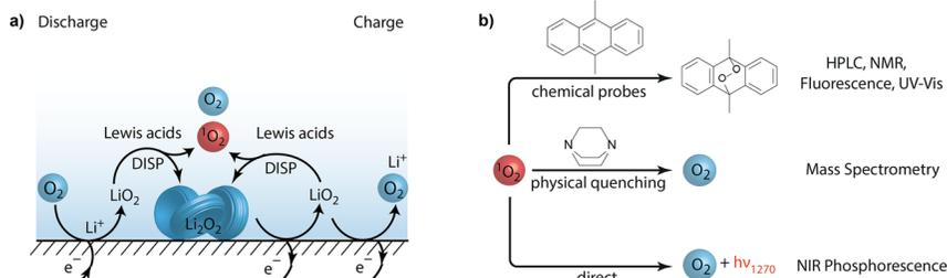
Fig. 1 (a) Superoxide disproportionation as the main source of  $^1\text{O}_2$  during charge and discharge of metal–air batteries. (b) Methods to detect singlet oxygen ( $^1\text{O}_2$ ) in non-aqueous oxygen redox systems.
