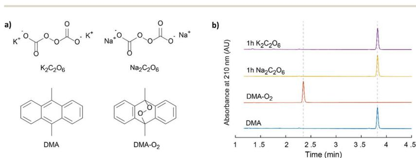
Fig. 3 (a) The structures of the symmetric Na and K peroxydicarbonates, DMA and DMA-O<sub>2</sub>. (b) HPLC elugrams of these peroxydicarbonates in contact with 30 mM DMA in DME together with reference elugrams of DMA and DMA-O<sub>2</sub>.
