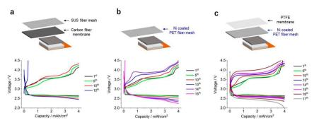
Fig. 4 Schematic illustration and discharge/charge profile of the LOB cells. (a) LOB cell equipped with a carbon fiber membrane as the gas-diffusion layer and an SUS fiber mesh as the current collector. (b) LOB cell equipped with a Ni-coated PET fiber mesh as the gas-diffusible current collector. (c) LOB cell equipped with a Ni-coated PET fiber mesh as the gas-diffusible current collector and a PTFE fiber membrane as the gas-diffusion layer.
