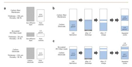
Fig. 5 Schematic illustration for quantitative information related to the electrolyte movement phenomenon. (a) Pore volume of the carbon electrode and gas-diffusion layer materials. (b) Estimation of electrolyte amount in cell A. (c) Estimation of electrolyte amount in cell B.
