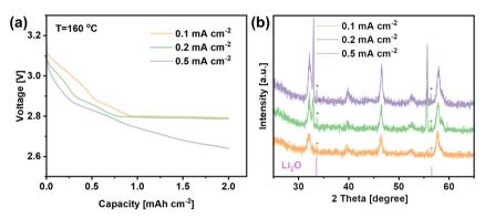
Fig. 5 (a) Discharge curves with a limited capacity of 2 mA h cm<sup>-2</sup> at 0.1, 0.2 and 0.5 mA cm<sup>-2</sup>. (b) XRD patterns of LNCO with the discharge product after being discharged at various current densities.
