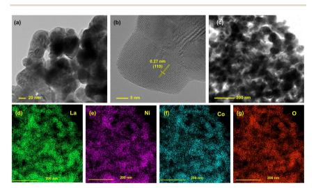
Fig. 2 (a) TEM image, (b) HR-TEM image, (c) area used for measuring the element distribution spectrum (EDS) and (d-g) corresponding EDS mapping images of the LNCO sample.
