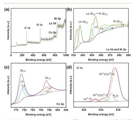
Fig. 3 (a) X-ray photoelectron spectroscopy (XPS) survey spectrum of LNCO. (b) XPS spectra of La 3d and Ni 2p in LNCO. (c) XPS spectra of Co 2p in LNCO. (d) XPS spectra of O 1s.
