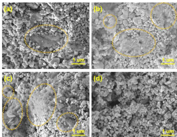
Fig. 6 SEM images of LNCO and the corresponding morphologies of the discharge product discharged at (a)  $0.1 \text{ mA cm}^{-2}$ , (b)  $0.2 \text{ mA cm}^{-2}$ , (c)  $0.5 \text{ mA cm}^{-2}$ , and (d) after the cycling test at  $0.5 \text{ mA cm}^{-2}$ .
