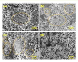
Fig. 6 SEM images of LNCO and the corresponding morphologies of the discharge product discharged at (a)  $0.1\,\mathrm{mA\,cm^{-2}}$ , (b)  $0.2\,\mathrm{mA\,cm^{-2}}$ , (c)  $0.5\,\mathrm{mA\,cm^{-2}}$ , and (d) after the cycling test at  $0.5\,\mathrm{mA\,cm^{-2}}$ .
