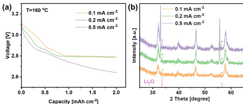
Fig. 5 (a) Discharge curves with a limited capacity of  $2 \text{ mA h cm}^{-2}$  at 0.1, 0.2 and  $0.5 \text{ mA cm}^{-2}$ . (b) XRD patterns of LNCO with the discharge product after being discharged at various current densities.
