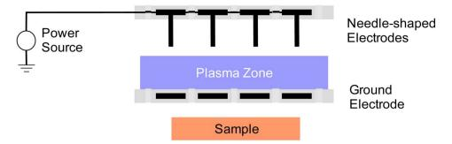
Scheme of a corona discharge plasma system with ground screen.
