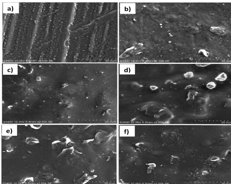
Fig. 4 SEM micrographs of PBAT/TKP blends: (a) PBAT, (b) PT-10, (c) PT-20, (d) PT-30, (e) PTG, and (f) PTP.
