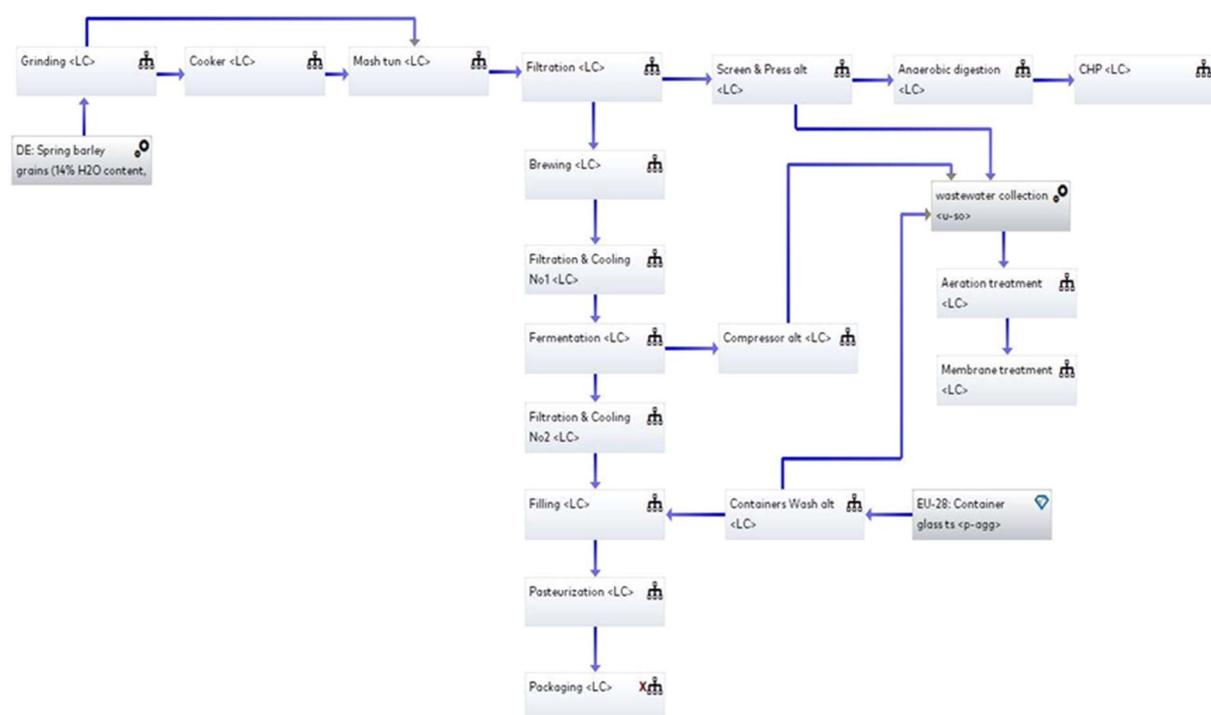
Fig. 2 Production processes and wastewater and solid waste treatment in Scenario A.
