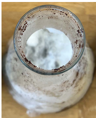
Fig. 1 Photo of the carob kibbles after 30 days of SSF in the Erlenmeyer flask.
