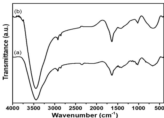
Fig. 4 Fourier transmission infrared spectroscopy (FTIR) spectra of (a) C-G and (b) BLCT-1.
