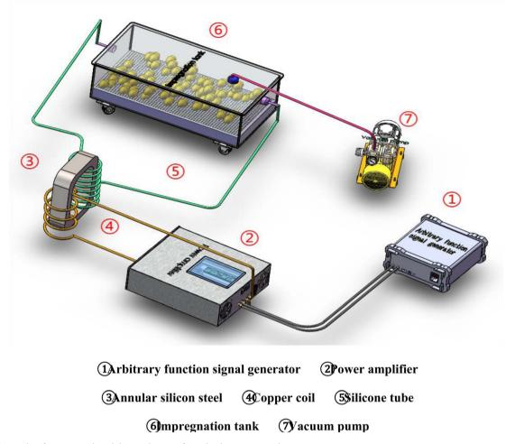
A schematic of magnetoelectricity equipment for salted egg processing
