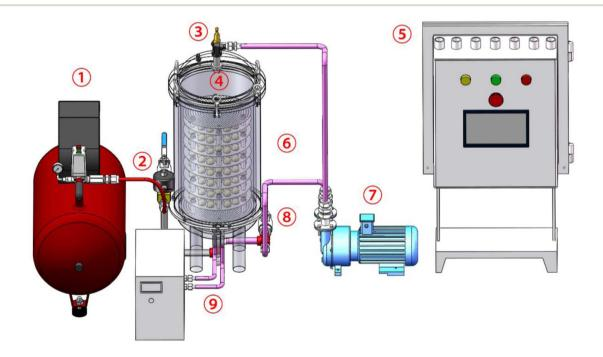
(1)Air compressor (2)Pressure adding electromagnetic valve
