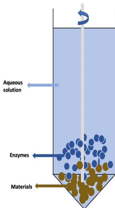
Fig. 5 Schematic representation of extraction assisted by enzymes.
