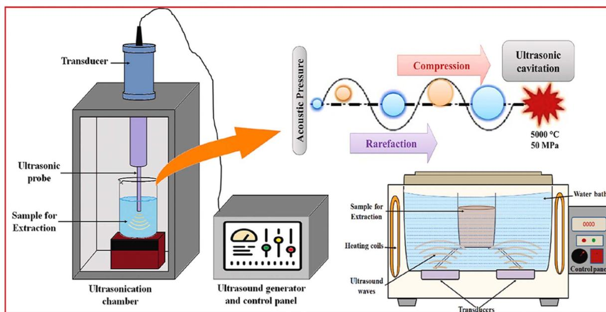
Fig. 6 Schematic representation of ultrasonic-assisted extraction (More *et al.*<sup>106</sup>).
