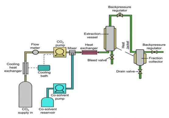
Fig. 4 Schematic representation of the supercritical CO<sub>2</sub> system coupled with co-solvent (Koubaa et al.<sup>97</sup>).
