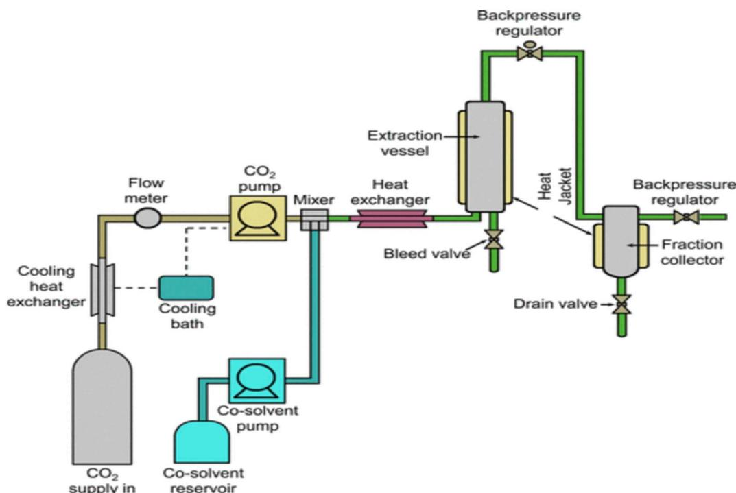
Fig. 4 Schematic representation of the supercritical CO<sub>2</sub> system coupled with co-solvent (Koubaa *et al.*<sup>97</sup>).
