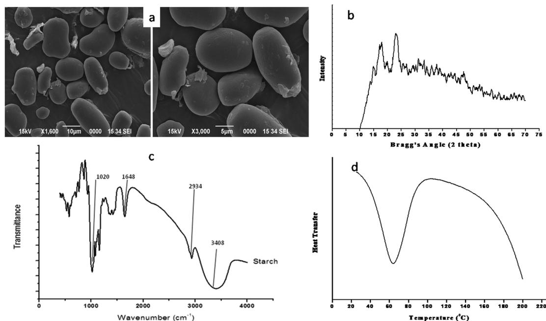
Fig. 2 Morphology and physical properties of water chestnut starch. (a) Scanning electron microscopy images of starch granules, (b) X-ray diffraction pattern, (c) FTIR spectra and (d) DSC thermogram.
