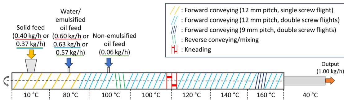
**Fig. 1** Extruder design and operating parameters for the extrusion process of composite high moisture meat alternatives. The feeding rates operated for the standard are underlined in red, the feeding rates for the emulsified oil samples are underlined in blue and the feeding rates for the non-emulsified oil samples are underlined in green.
