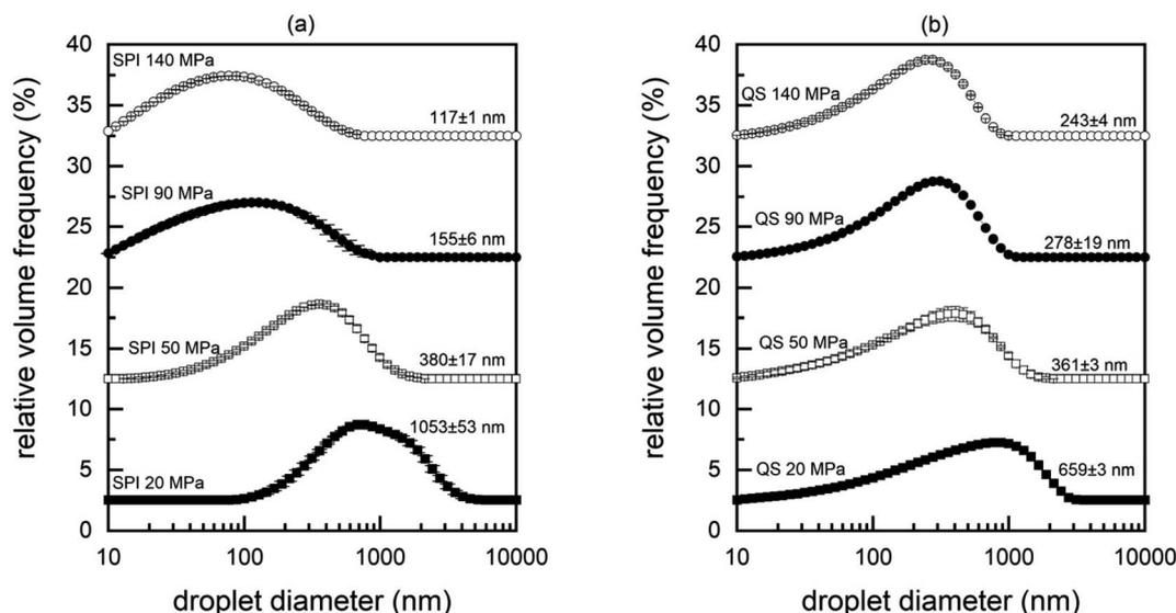
Fig. 2 Volume-based particle size distribution and the corresponding mean particle size  $d_{4,3}$  of emulsions homogenized at four different pressures (20, 50, 90 & 140 MPa) and stabilized by soy protein isolate (SPI) addition (a) and *Quillaja* saponin (QS) addition (b), respectively.
