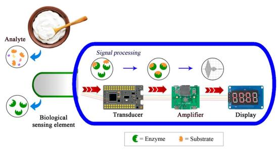
Fig. 1 Schematic diagram illustrating biosensor operation principles, highlighting recognition element-analyte interaction and signal transduction.
