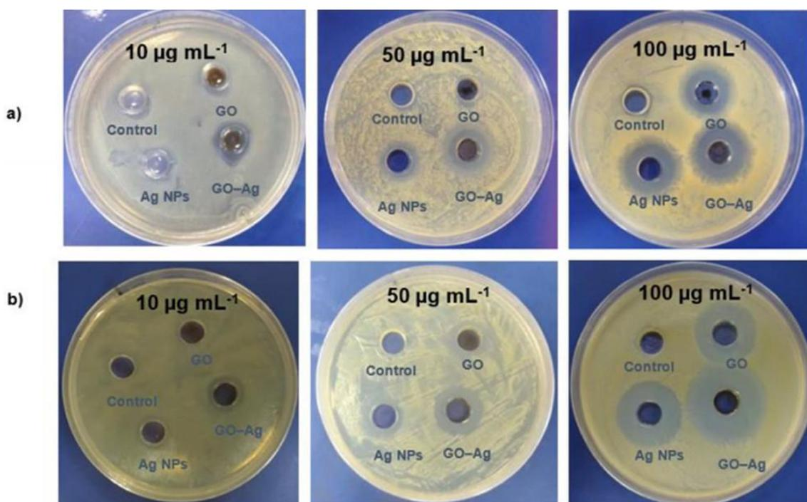
Fig. 17 Zone of inhibitions displayed by control, GO, Ag NPs, and GO-Ag against (a) *E. coli* and (b) *S. aureus*.<sup>110</sup>
