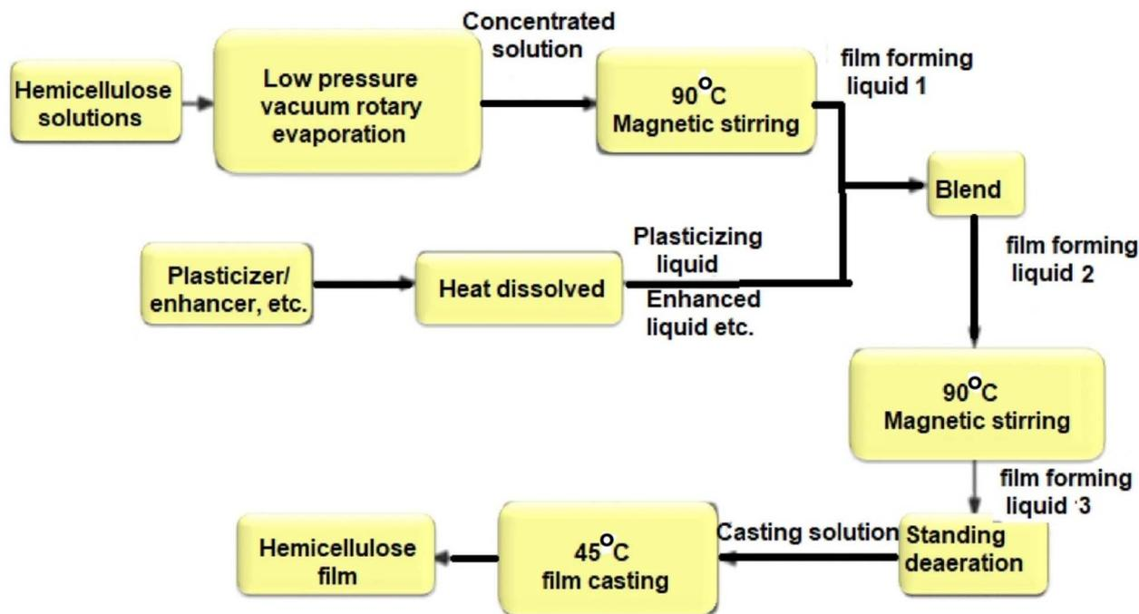
Fig. 11 Flow chart of hemicellulose film formation.<sup>39</sup> Reproduced (adapted) with permission from ref. 39. Copyright [2022] [Springer Nature].
