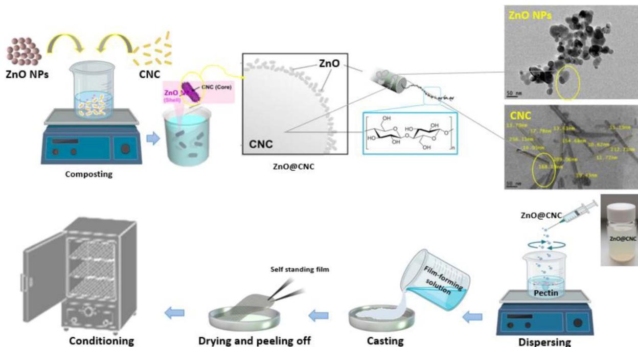
Fig. 55 Schematic diagram for the preparation of ZnO/CNC composite and pectin-based nanocomposite films.<sup>395</sup>
