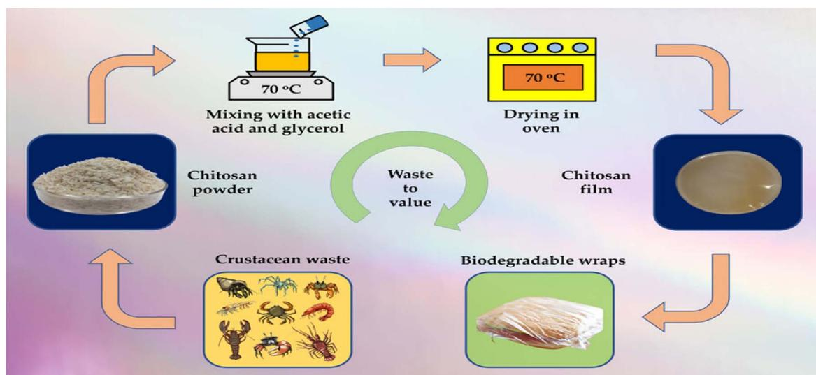
Fig. 44 Schematic representation of synthesis and use of glycerol-added chitosan films for food packaging.<sup>384</sup> Reproduced (adapted) with permission from ref. 384. Copyright [2023] [ACS].
