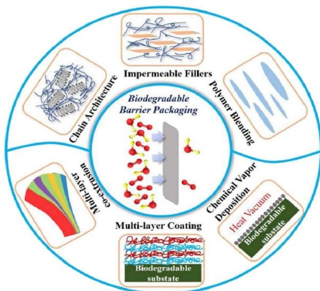
Fig. 39 High barrier biodegradable packaging approaches.<sup>355</sup> Reproduced (adapted) with permission from ref. 355. Copyright [2021] [Elsevier].
