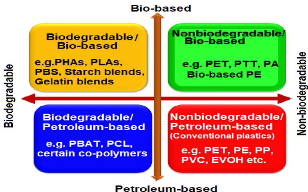
Fig. 5 Different types of polymer packaging materials.<sup>33</sup> Reproduced (adapted) with permission from ref. 33. Copyright [2020] [Elsevier].
