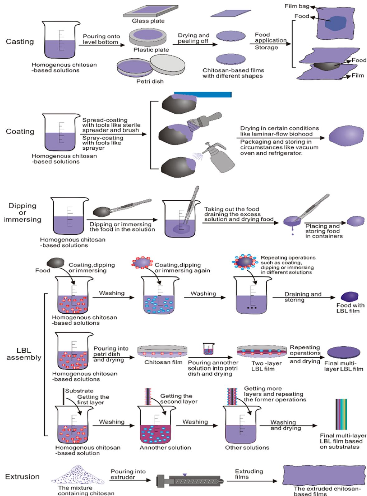
Fig. 28 Different methods of fabrication of chitosan-based films.<sup>197</sup> Reproduced (adapted) with permission from ref. 197. Copyright [2013] [Elsevier].
