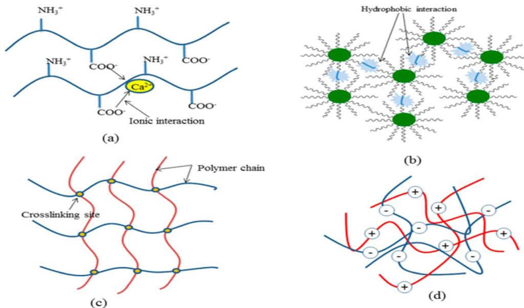
Fig. 32 Different polymerization techniques for the synthesis of hydrogels: (a) ionic interaction, (b) hydrophobic interaction, (c) cross-linking junction by cooling, and (d) complex coacervate.<sup>329</sup> Reproduced (adapted) with permission from ref. 329. Copyright [2018] [ACS].
