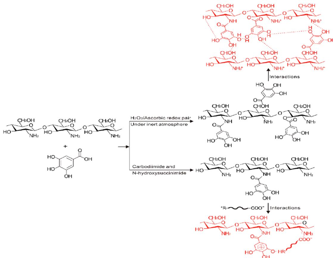
Fig. 24 Grafting of gallic acid onto chitosan.<sup>196</sup> Reproduced (adapted) with permission from ref. 196. Copyright [2014] [ACS].
