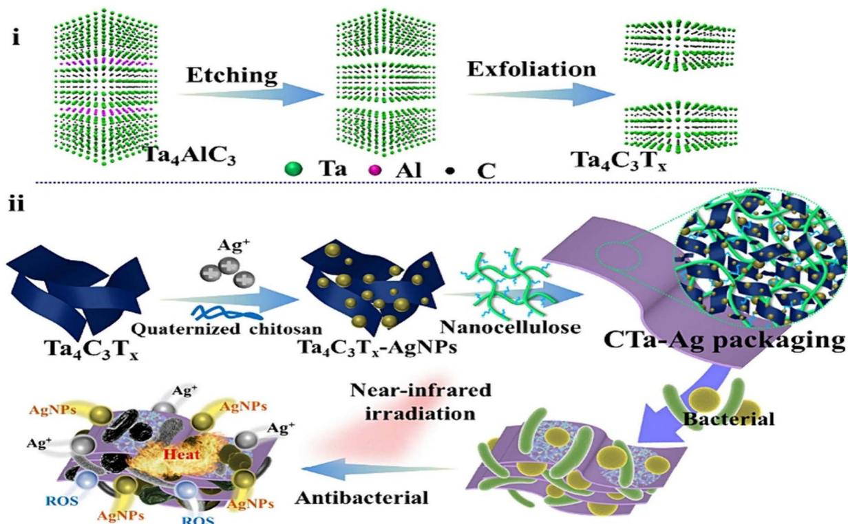
Fig. 54 Schematic illustration of (i)  $Ta_4C_3T_x$  preparation from  $Ta_4AlC_3$ , and (ii) fabrication of CTa-Ag packaging.<sup>394</sup> Reproduced (adapted) with permission from ref. 394. Copyright [2024] [Elsevier].
