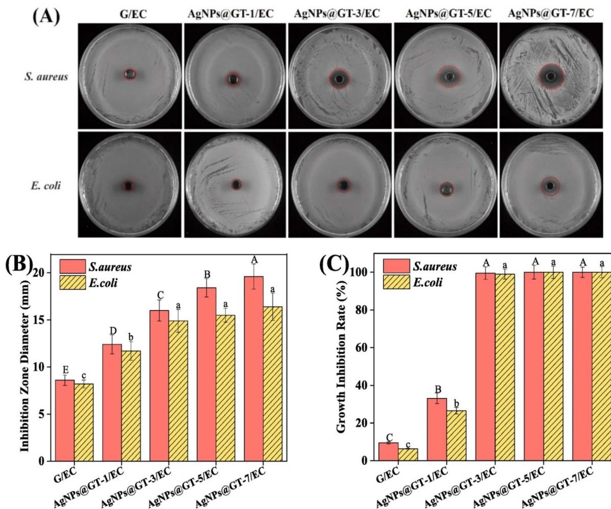
Fig. 51 Antibacterial activities of different film samples against *S. aureus* and *E. coli*: (A) antibacterial photographs, (B) inhibition zone diameter and (C) growth inhibition rate.<sup>391</sup> Reproduced (adapted) with permission from ref. 391. Copyright [2024] [Elsevier].
