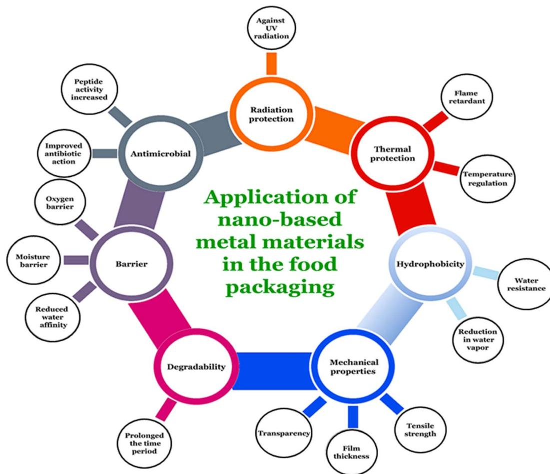
Fig. 19 Applications and characteristics of nano-based metal-materials in food packaging.<sup>118</sup>
