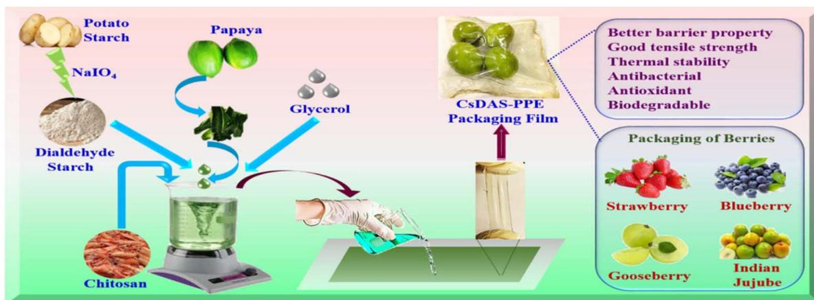
Fig. 49 Diagrammatic depiction of the fabrication of chitosan (Cs)-dialdehyde starch (DAS) Schiff base hydrogels containing *C. papaya* peel extract (CsDAS-PPE hydrogel) as novel packaging materials for fresh berries.<sup>389</sup>
