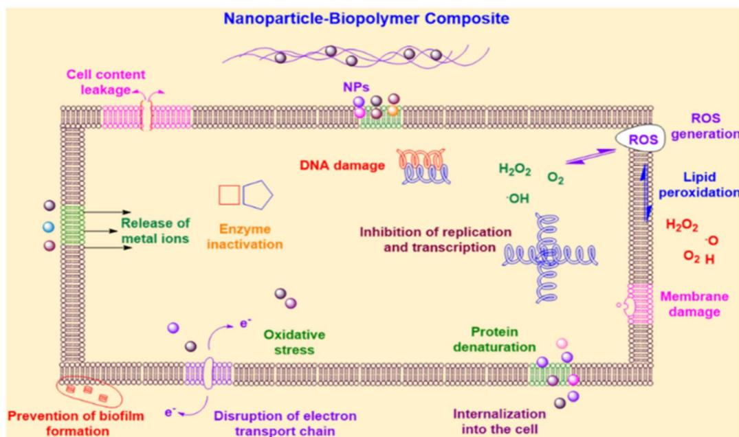
Fig. 14 Antimicrobial mechanisms of action of nanocomposites designed for food packaging.<sup>96</sup>
