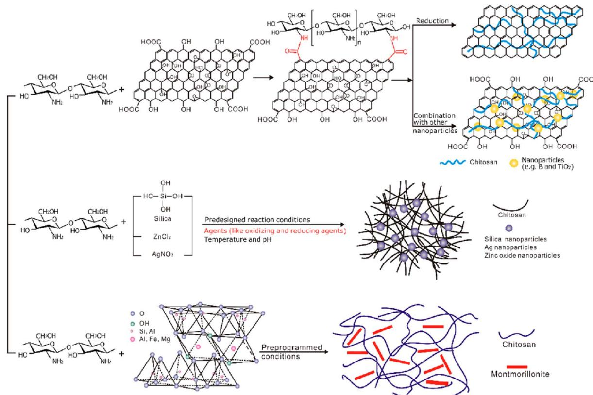
Fig. 26 Preparation of chitosan–inorganic complexes.<sup>197</sup> Reproduced (adapted) with permission from ref. 197. Copyright [2013] [Elsevier].
