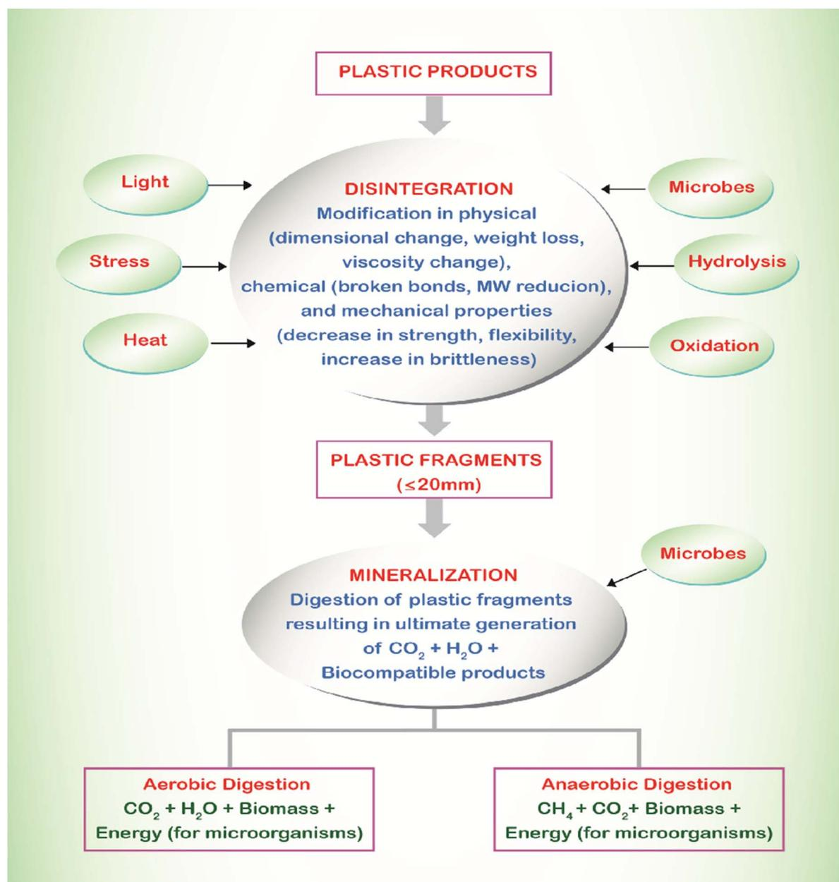
Fig. 35 Schematic representation of plastic degradation.<sup>346</sup> Reproduced (adapted) with permission from ref. 346. Copyright [2006] [Elsevier].
