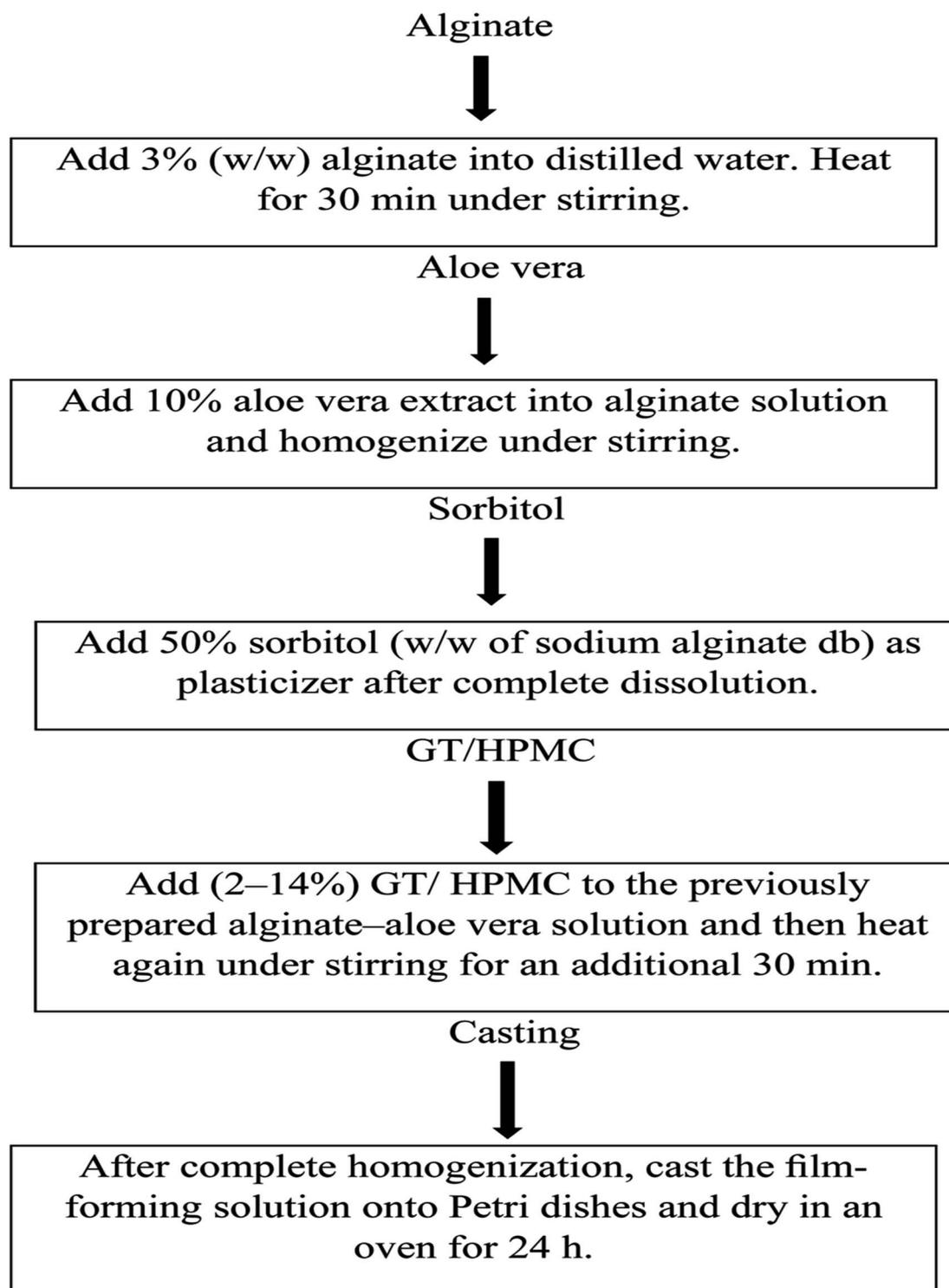
Fig. 48 Flow diagram showing the preparation of the alginate–Aloe vera films.<sup>388</sup>
