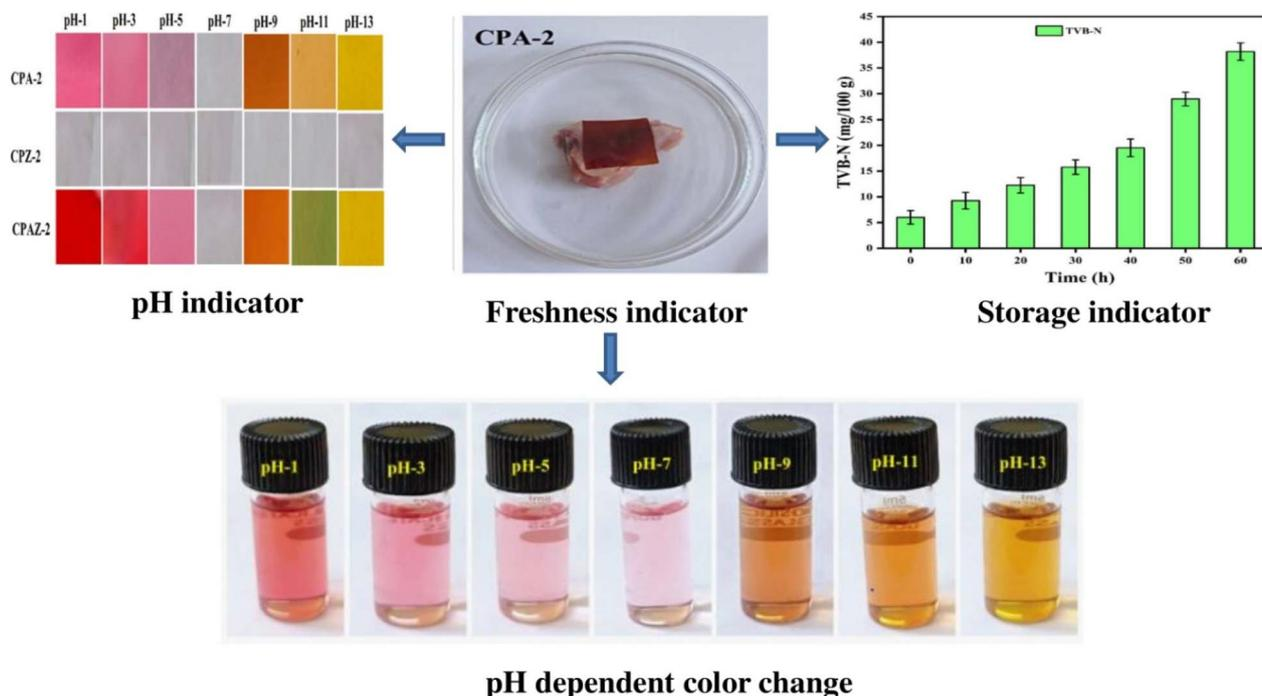
Fig. 47 Schematic representation of the use of bionanocomposite films based on chitosan/polyvinyl alcohol with ZnO NPs and *Carissa carandas* extract anthocyanin for smart packaging materials.<sup>387</sup> Reproduced (adapted) with permission from ref. 387. Copyright [2023] [ACS].
