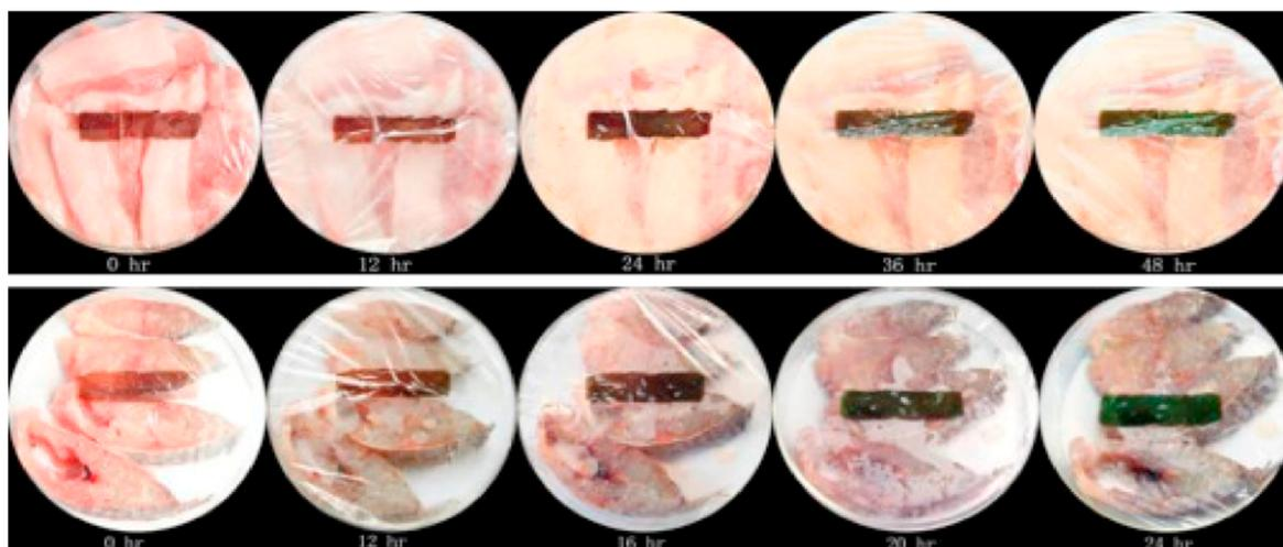
Fig. 30 Sensing film application as a sticker sensor for pork & fish freshness.<sup>311</sup> Reproduced (adapted) with permission from ref. 311. Copyright [2014] [Elsevier].
