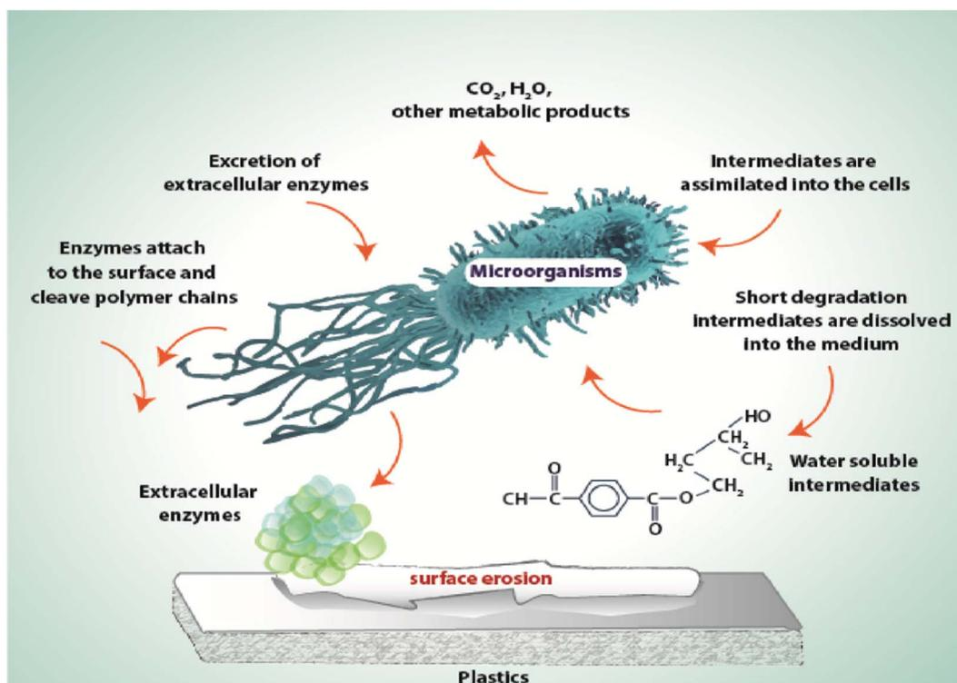
Fig. 36 General mechanism of plastic degradation under aerobic conditions.<sup>347</sup> Reproduced (adapted) with permission from ref. 347. Copyright [2005] [John Wiley and Sons].
