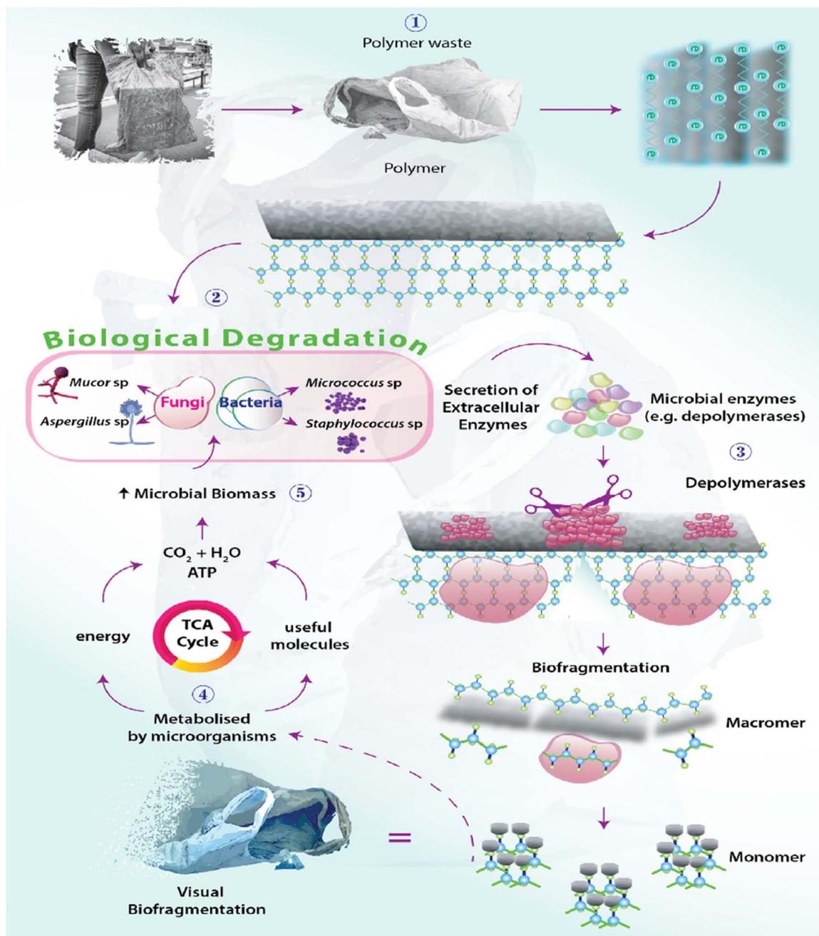
Fig. 40 Biodegradation of polyethylene.<sup>360</sup> Reproduced (adapted) with permission from ref. 360. Copyright [2021] [Elsevier].
