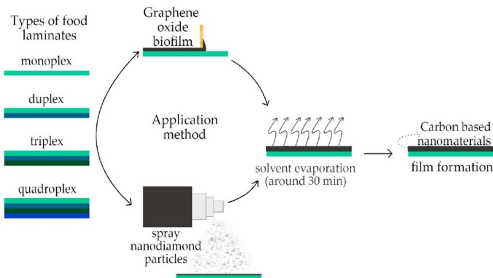
Fig. 18 Schematic representation of the carbon based nanomaterials film formation.<sup>117</sup>
