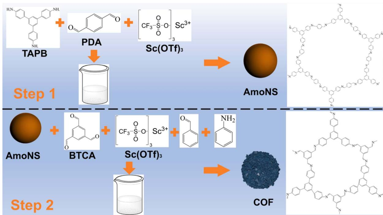
Fig. 52 The synthesis mold of AmoNS and COFs.<sup>392</sup> Reproduced (adapted) with permission from ref. 392. Copyright [2023] [Elsevier].
