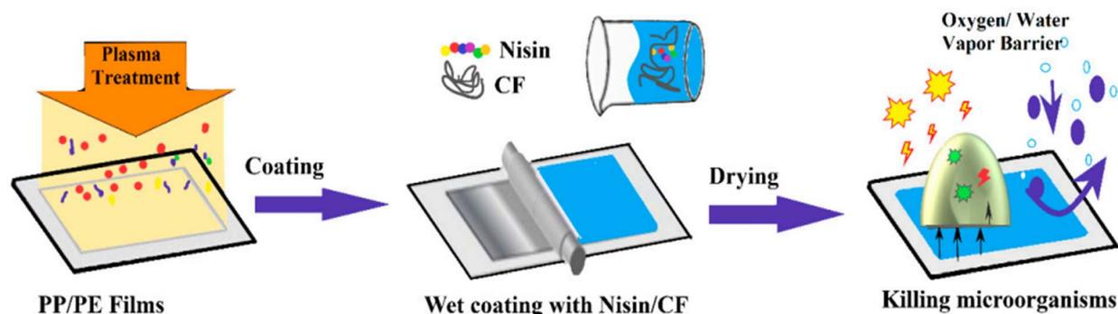
Fig. 21 Coating of polypropylene/polyethylene (PP/PE) films with other polymers (cellulose fibers—CF) and loading with antibacterial agents (nisin).<sup>152</sup>
