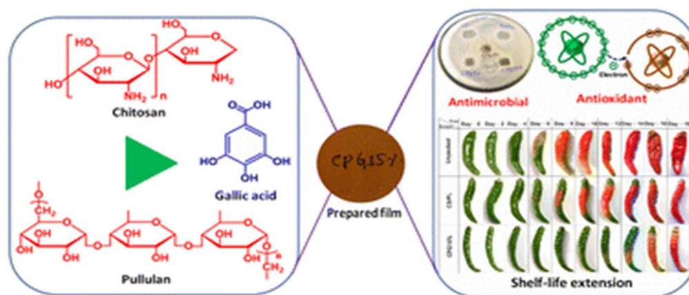
Fig. 50 Gallic acid functionalized chitosan/pullulan active bio-films for the preservation and shelf-life extension of green chillies. 390
