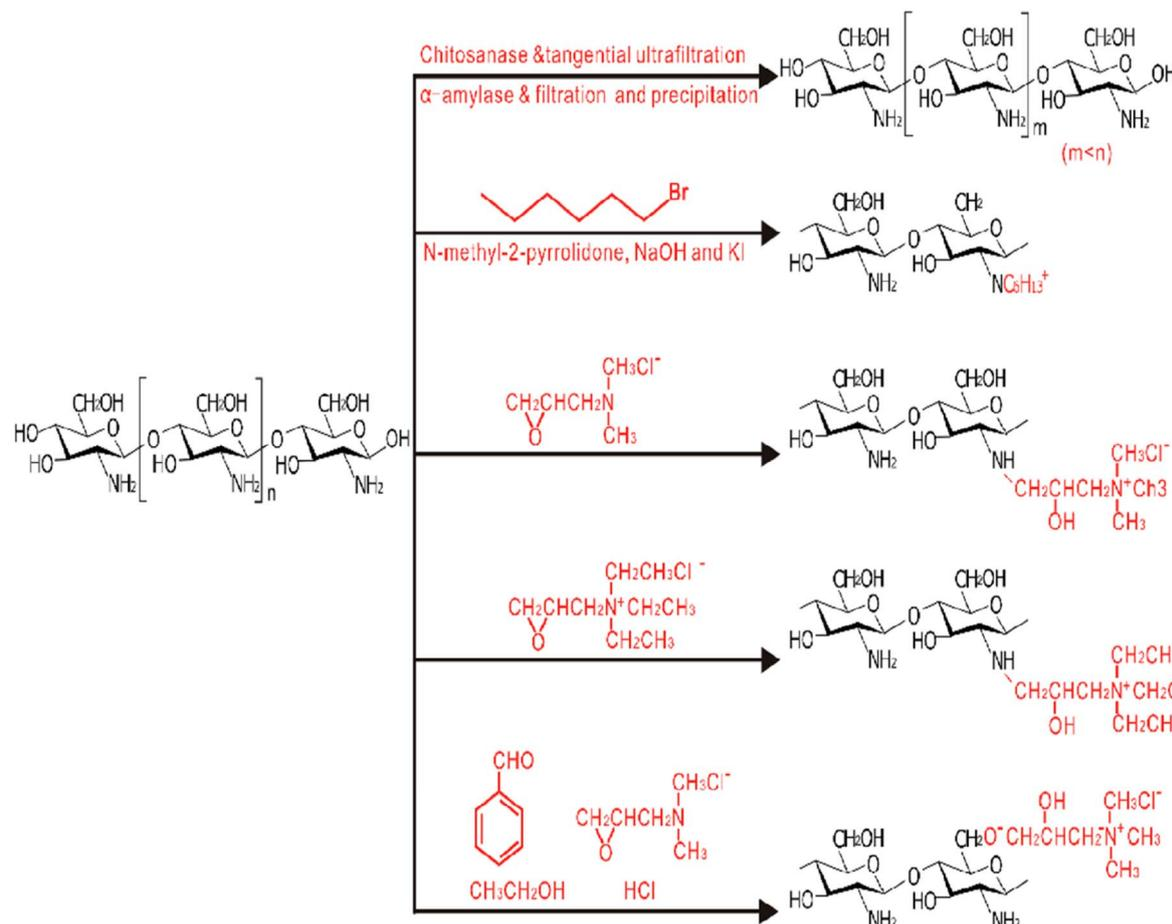
Fig. 27 Chitosan derivative development of fabrication of chitosan/chitosan derivatives-based films.<sup>197</sup> Reproduced (adapted) with permission from ref. 197. Copyright [2013] [Elsevier].
