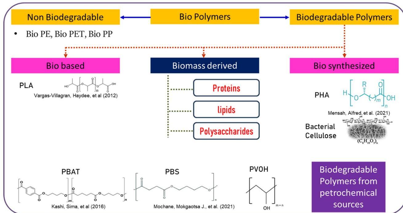
Fig. 8 Detailed classification of biopolymers based on biodegradability with some examples and other biodegradable polymers that are sourced from petrochemicals with structural representations.
