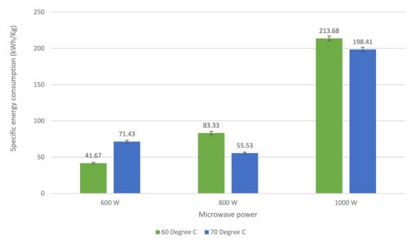
Fig. 2 Specific energy consumption of microwave-dried shrimp.
