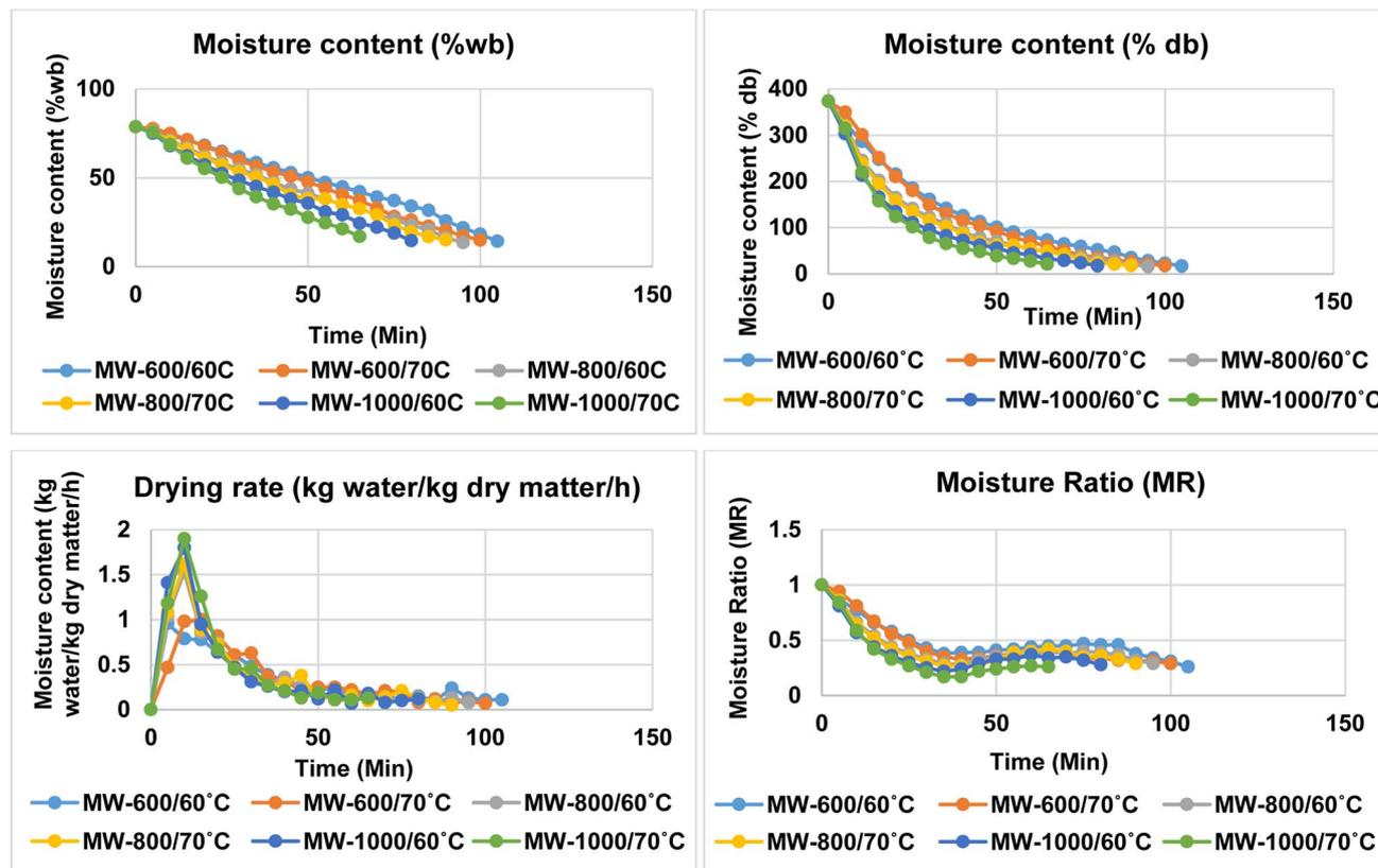
Fig. 1 Drying kinetics of microwave-dried shrimp.
