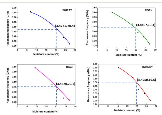
Resonance frequency with respect to moisture content corresponding to grain powder samples.
