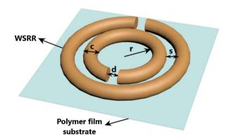
Fig. 1 WSRR structure fixed on a thin polymer film substrate and having structural parameters – inner radius (r), metal width (c), split gap (d) and gap between the rings (s).
