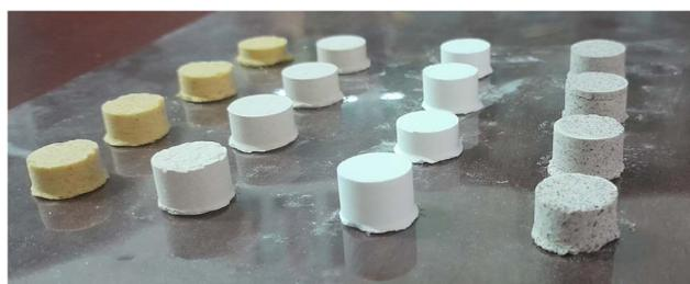
Fig. 3 The compacted dry flour samples of corn, wheat, barley and ragi (from left to right).
