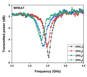
Fig. 8 Transmitted power with the frequency of the WSRR corresponding to compacted dry wheat powder samples.
