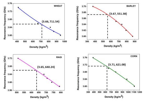
Resonance frequency with respect to density corresponding to dry powder samples.
