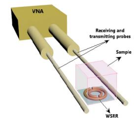
Fig. 2 Schematic representation of the dielectric characterization setup including the WSRR structure with a dielectric sample placed on its upper surface and the measuring device VNA
