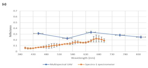
Fig. 12 Comparison of spectral profile in reflectance between multispectral UAV (blue) and multiwavelength spectral ground reference data using a Spectro-1 spectrometer (orange) across three growth stages of oats. (a) June (Stage 3 – flowering), (b) July (Stage 4 – grain filling), and (c) August (Stage 5 - ripening)
