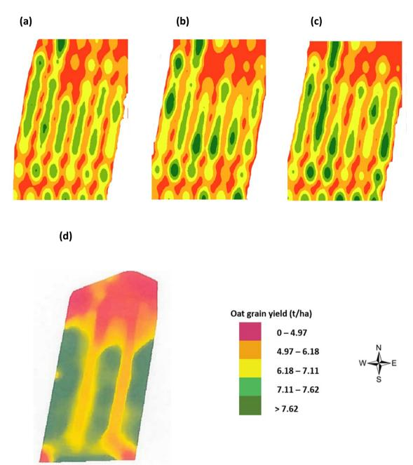
Fig. 15 Oats grain yield maps by KDE (a) actual yield as measured in laboratory (in August), (b) estimated yield by NDVI (in June), (c) estimated yield by CI green VI (in June), and (d) from on-board combine harvester yield monitor (FarmTRX system) (in August).
