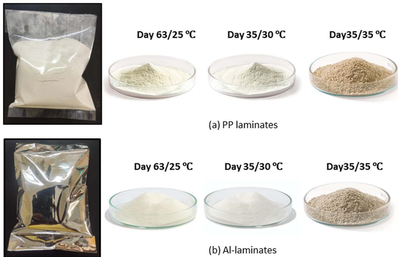
Fig. 7 Physical appearance of synbiotic KMB powder by the end of shelf-life at both the storage temperatures for both the packaging materials (a) PP laminates and, (b) Al-laminates.
