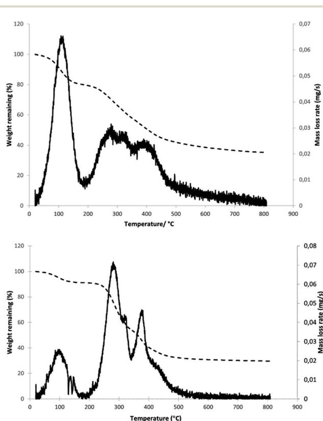
Fig. 6 TG data for a sample of peat (top) and SCG (bottom). Dashed lines show remaining weight (in %) plotted against temperature (°C). Continuous lines show mass loss rate ( $\text{mg s}^{-1}$ ) against temperature (°C).
