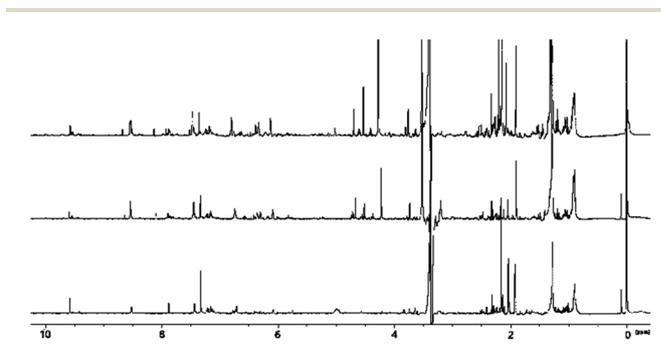
Fig. 5 Comparison of <sup>1</sup>H NMR spectra (recorded at 400 MHz) of methanolic solutions treated with peat smoke (bottom), spent caffeinated coffee grounds smoke (middle) and SCG from decaffeinated coffee smoke (top).
