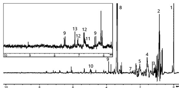
Fig. 2 <sup>1</sup>H NMR spectrum of a methanol extract of peat recorded at 400 MHz. (1) TSP reference; (2) fatty acids, alcohols, alkanes, alkenes (methylene groups); (3) ethylphenol; (4) fatty acids, alcohols, alkanes, alkenes (methyl groups); (5) acetic acid; (6) acetone; (7) *o*-cresol, *p*-cresol; (8) methanol; (9) ferulic acid; (10) water, methanol (OH group); (11) *o*-cresol; (12) *o*-cresol, *p*-cresol, ferulic acid; (13) syringol.
