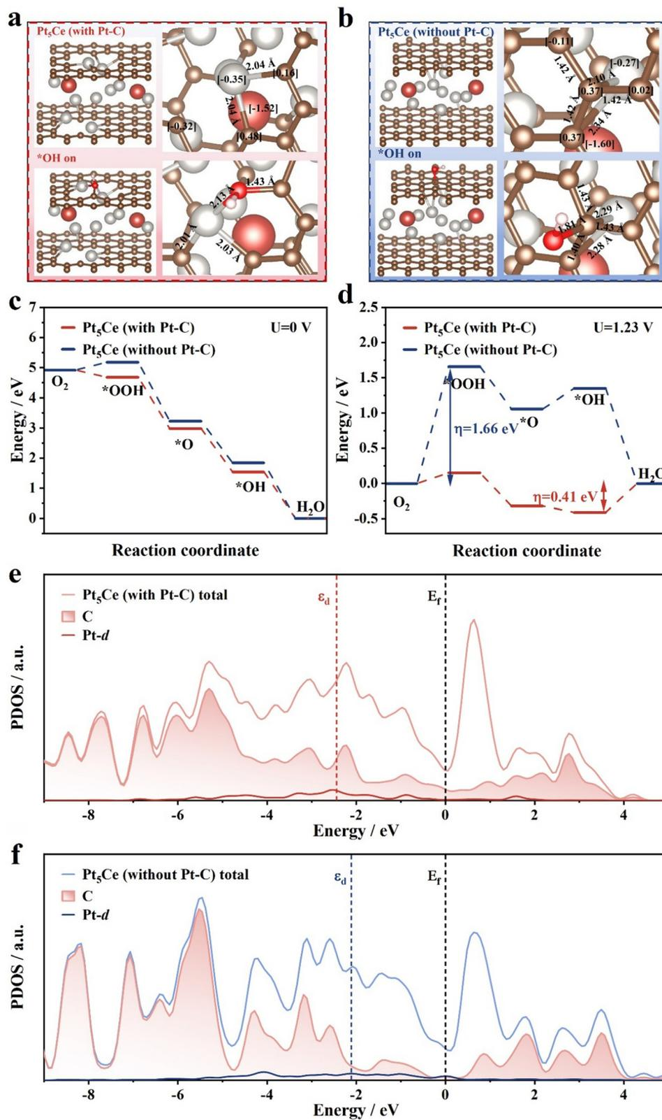
Fig. 5 DFT calculation results. The models of initial state, with adsorbed OH intermediates on, and Bader charge of (a) Pt<sub>5</sub>Ce (with Pt-C) and (b) Pt<sub>5</sub>Ce (without Pt-C). Gibbs free energy profile of the ORR process at (c)  $U = 0$  V and (d)  $U = 1.23$  V. The PDOS results of (e) Pt<sub>5</sub>Ce (with Pt-C) and (f) Pt<sub>5</sub>Ce (without Pt-C).
