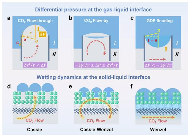
Fig. 3 Schematic illustration of differential pressure at the gas-liquid interface and corresponding (a) CO<sub>2</sub> flow-through, (b) CO<sub>2</sub> flow-by and (c) GDE flooding modes. Wetting dynamics at the solid-liquid interface including (d) Cassie state, (e) Cassie-Wenzel coexistence state, and (f) Wenzel state.
