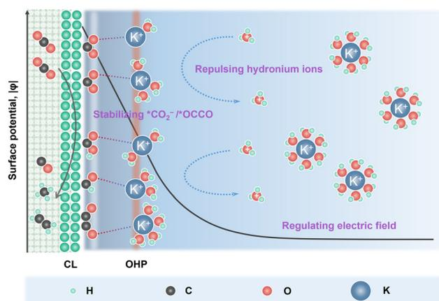
Fig. 1 Schematic illustration of the alkali cation effects in acidic eCO<sub>2</sub>R.
