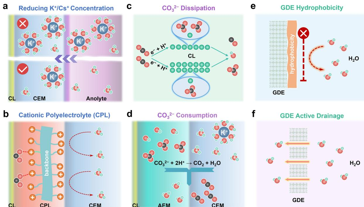
Fig. 4 Remedies of mitigating salt precipitation and water flooding in acidic eCO<sub>2</sub>R MEAs including (a) reducing K<sup>+</sup>/Cs<sup>+</sup> concentration in anolytes, (b) replacing K<sup>+</sup>/Cs<sup>+</sup> with a cationic polyelectrolyte layer (CPL), (c) CO<sub>3</sub><sup>2-</sup> dissipation in the catalyst layer (CL), (d) accelerating CO<sub>3</sub><sup>2-</sup> consumption, (e) tailoring GDE hydrophobicity, and (f) GDE active drainage.
