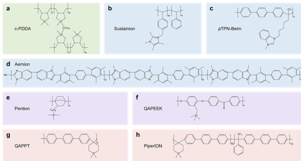
Fig. 5 Molecular structures of AEMs/AEIs that are feasible in eCO<sub>2</sub>R electrolyzers fed with pure acid or pure water, including (a) c-PDDA, (b) Sustainion, (c) pTPN-Beim, (d) Aemion, (e) Pention, (f) QAPEEK, (g) QAPPT and (h) PiperION.
