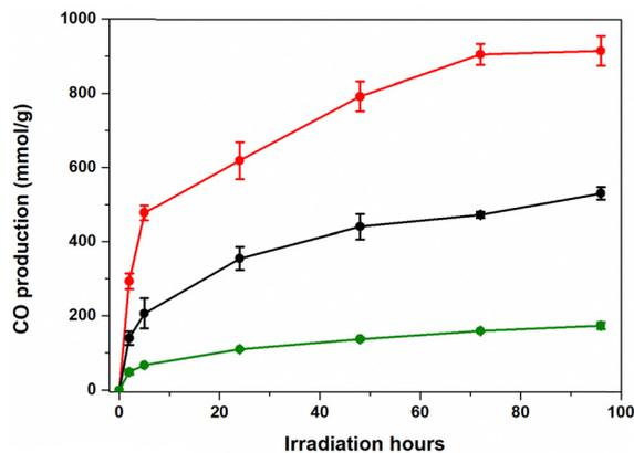
Fig. 4 Photocatalytic CO<sub>2</sub>-to-CO conversion activities of ZnP@TiO<sub>2</sub> NPs in 4 mL ACN solution containing 50 mM of BIH; (black): 0.12 μmol (0.1 mg) of PS, 0.032 μmol (0.05 mg) of Fe(o-TMA), (red): 0.12 μmol (0.1 mg) of PS, 0.032 μmol (0.05 mg) of Fe(o-TMA) and 0.1 M of phenol, (green): 0.12 μmol (0.1 mg) of PS (0.1 mg), 0.016 μmol (0.025 mg) of Fe(o-TMA) and 0.1 M of phenol. The reported values are the average of three independently repeated experiments.
