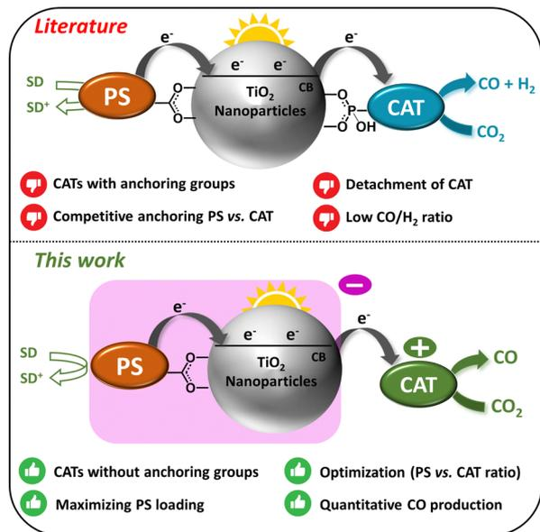
Fig. 1 DSPs for CO<sub>2</sub>-to-CO reduction: (upper panel) previous examples from the literature; (lower panel) our strategy comprising a positively-charged molecular catalyst (CAT) and negatively-charged TiO<sub>2</sub> nanoparticles (PS–TiO<sub>2</sub> NPs).
