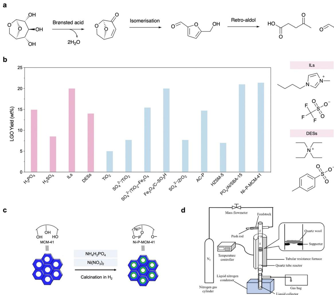
**Fig. 3** (a) Reaction scheme of LGA-to-LGO process and production of side-products. (b) Performance comparison of previously reported catalysts for LGO production in cellulose pyrolysis and molecular structures of ILs and DESs as representative of homogeneous catalysts (selected from the highest yield achieved under ambient conditions).<sup>21</sup> (c) Modification of MCM-41 for cellulose CFP.<sup>31</sup> (d) Reaction set-up for cellulose CFP to produce LGO.<sup>32</sup>
