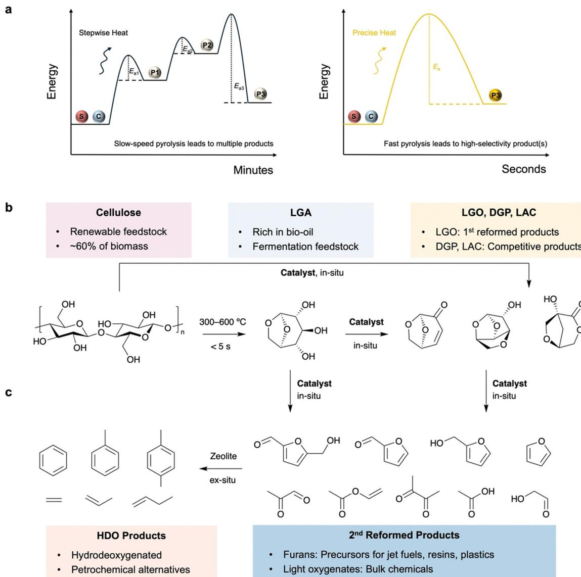
**Fig. 1** (a) Schematic illustration of reaction progress in slow pyrolysis and fast pyrolysis. Reaction scheme of cellulose CFP to produce (b) anhydrous sugars and (c) furans, light oxygenates and aromatics (catalysts to be discussed are in bold font).
