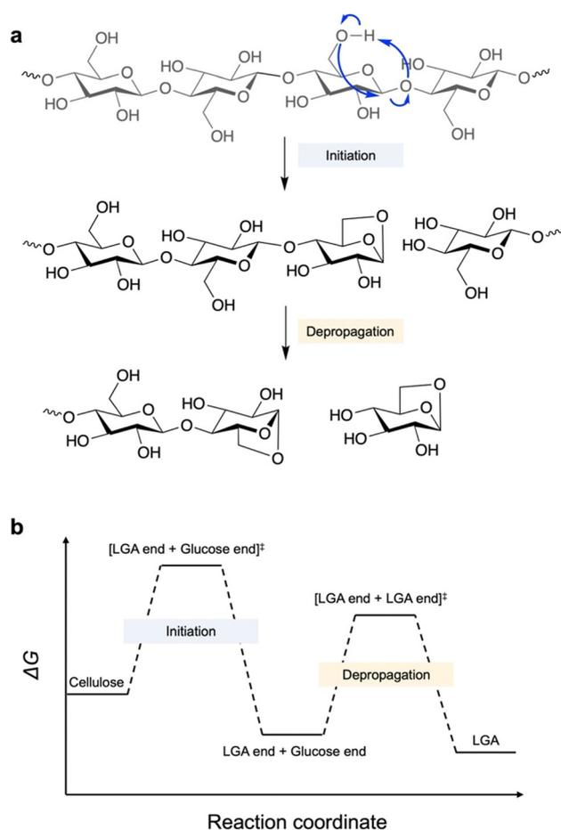
Fig. 2 (a) Reaction scheme of cellulose depolymerisation to release LGA in pyrolysis. (b) Free energy change of key steps in cellulose depolymerization.<sup>15</sup>
