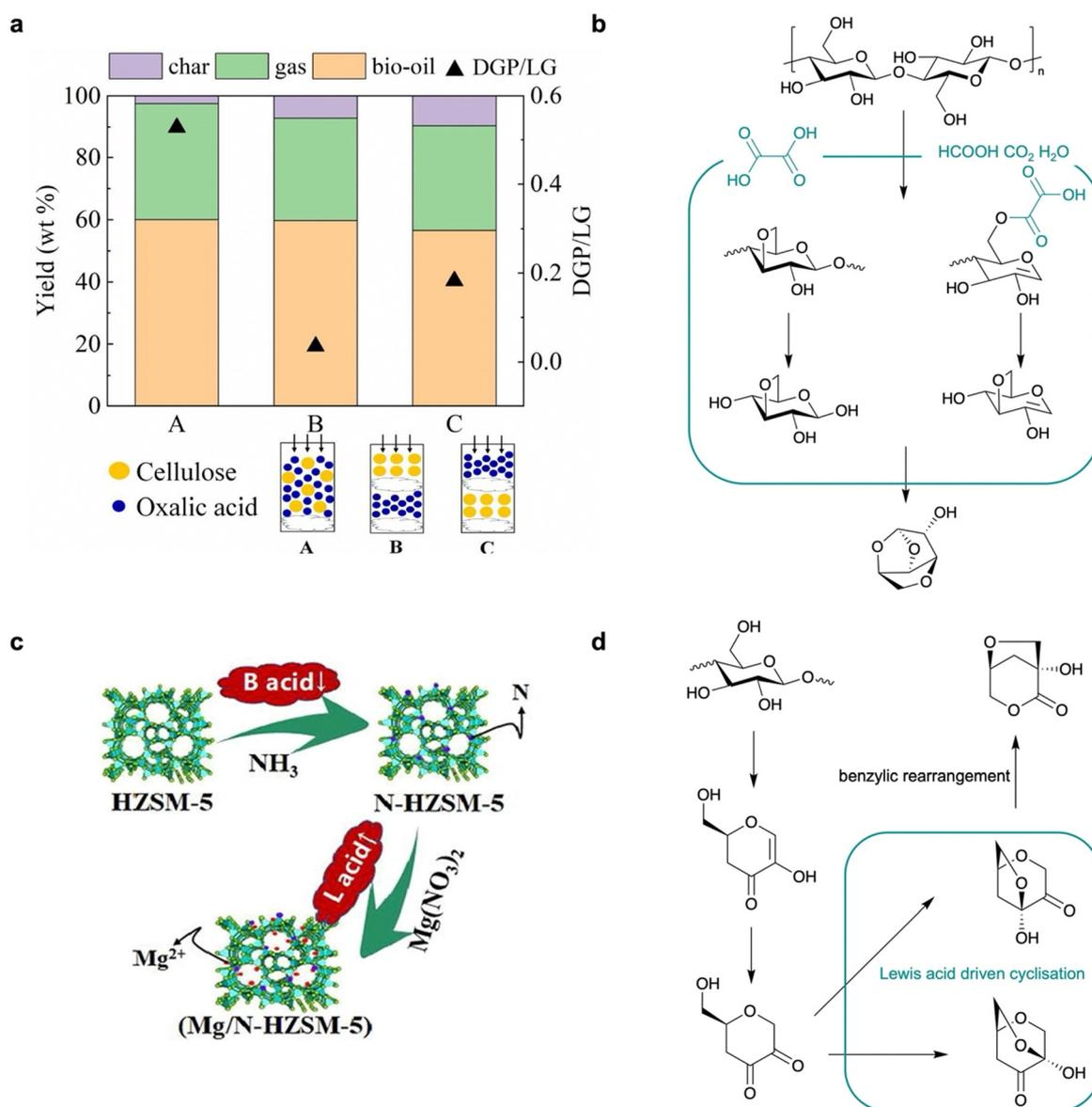
Fig. 4 (a) Performance comparison of cellulose CFP with oxalic acid to produce DGP in different loading set-ups.<sup>18</sup> (b) Reaction pathway of cellulose CFP to produce DGP. (c) Modification of HZSM-5 for cellulose CFP.<sup>40</sup> (d) Reaction pathway of cellulose CFP to produce LAC.
