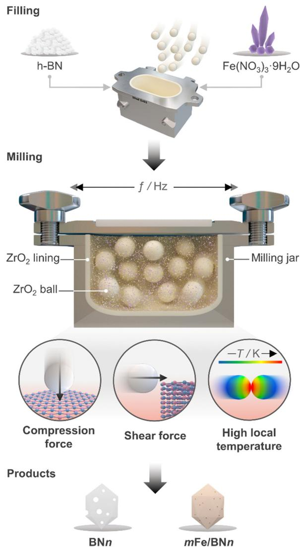
Fig. 1 Schematic representation of the milling jar used for preparation of  $m\text{Fe}/\text{BN}_n$  ( $m$  = metal content in wt% and  $n$  = milling time in h) catalysts via ball milling and the associated mechanophysical processes occurring during the milling process.
