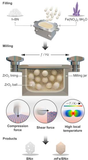
Fig. 1 Schematic representation of the milling jar used for preparation of mFe/BNn (m = metal content in wt% and n = milling time in h) catalysts via ball milling and the associated mechanophysical processes occurring during the milling process.
