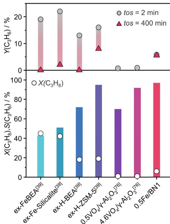
Fig. 6 N<sub>2</sub>O-ODHP performance, expressed in terms of C<sub>3</sub>H<sub>8</sub> conversion, C<sub>3</sub>H<sub>6</sub> selectivity and yield, of benchmark catalysts reported in the literature. The reaction conditions are provided in Table S3 (ESI†).
