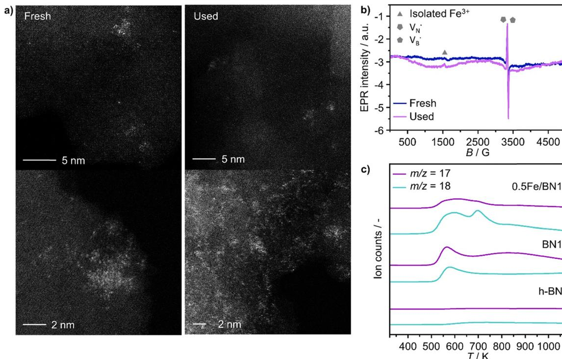
Fig. 5 Characterization of 0.5Fe/BN1 before and after use in  $\text{N}_2\text{O}$ -ODHP for 18 h. (a) High resolution HAADF-STEM micrographs and (b) EPR spectra acquired at 293 K of 0.5Fe/BN1 after the reaction. (c)  $\text{NH}_3$ -TPD of as prepared 0.5Fe/BN1 and BN supports.
