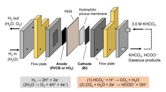
Fig. 1 Schematics of a bicarbonate-fed electrolyzer, wherein aqueous  $HCO_3^-$  reacts with  $H^+$  near the proton exchange membrane (PEM) to produce  $CO_2$  (eqn (1)), which is electrocatalytically reduced to formate on the Bi cathode (eqn (2)). A hydrophilic porous membrane between PEM and the cathode facilitates *in situ*  $CO_2$  generation. Pt/CB or  $IrO_2$  anodes are used for hydrogen oxidation and oxygen evolution reactions, respectively.
