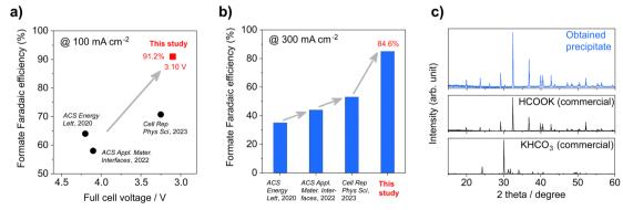
Fig. 6 Comparison of performances with literature on bicarbonate electrolyzers for formate synthesis: (a) formate FE and full cell voltage at 100 mA cm<sup>-2</sup> and (b) formate FE at 300 mA cm<sup>-2</sup> (except for *Cell Rep. Phys. Sci.*, 2023 at 200 mA cm<sup>-2</sup>). (c) Powder XRD patterns of the precipitate obtained by evaporating the catholyte after the bicarbonate electrolyzer reaction (Fig. S10, ESI†) and commercial salts of HCOOK and KHCO<sub>3</sub>.
