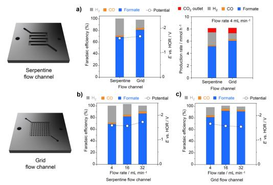
Fig. 4 (a) Influence of liquid flow channels on FEs of each product, full-cell potential (vs. HOR), production rate, and CO<sub>2</sub> outlet rate under 3.0 M KHCO<sub>3</sub> flow at 4 mL min<sup>-1</sup>. Flow rate dependence on performances using flow field plates with (b) serpentine channel (width/depth: 2 mm) and (c) grid channel (width/depth: 1 mm). Electrocatalytic reactions were performed at 100 mA cm<sup>-2</sup> with the intermediate cellulose esters membrane.
