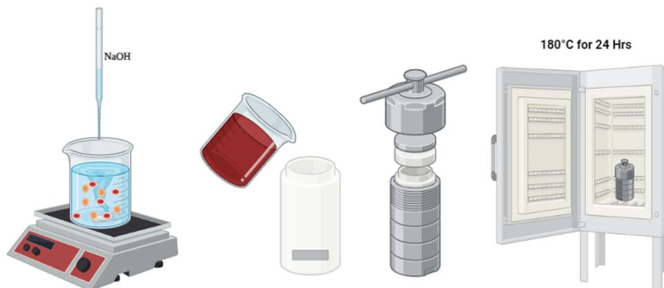
Scheme 1 Hydrothermal synthesis of the  $\text{CoFe}_2\text{O}_4/\text{Ni}$  foam electrodes.
