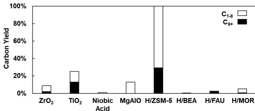
Fig. 1 Screening catalysts for 4-heptanone upgrading. C<sub>9+</sub> products are desired for jet applications. Reaction conditions:  $T$ : 350 °C,  $P_{\text{Total}}$  = 150 kPa,  $P_{4\text{-Heptanone}}$  = 15 kPa, balance He (30 sccm), WHSV = 1 h<sup>-1</sup>,  $m_{\text{catalyst}}$  = 1 g.
