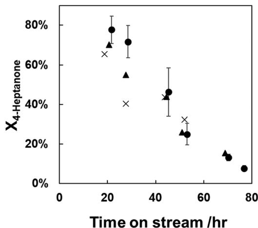
Fig. 4 Deactivation trends in 4-heptanone upgrading over H/ZSM-5 during repeated experiments with intervening catalyst regenerations. Reaction conditions:  $T$ : 350 °C,  $P_{\text{Tot}}$  = 140–160 kPa,  $\text{WHSV}$  = 3.1–3.6  $\text{h}^{-1}$ ,  $m_{\text{catalyst}}$  = 0.27–0.31 g. ●: fresh catalyst (0.30 g); ×: once-regenerated catalyst (0.31 g); ▲: twice-regenerated catalyst (0.27 g). Error bars are standard deviations of three independent runs on fresh catalysts.
