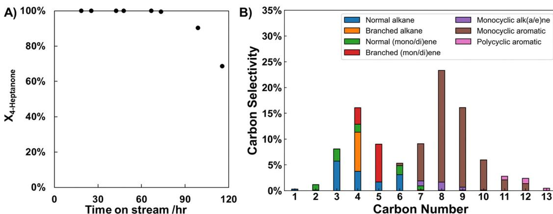
Fig. 2 (A) 4-Heptanone conversion ( $X_{4\text{-heptanone}}$ ) over time and (B) product selectivities at full conversion in 4-heptanone upgrading over H/ZSM-5 (Si/Al = 40). Reaction conditions:  $T$  = 350 °C,  $P_{\text{Total}}$  = 140 kPa,  $P_{4\text{-Heptanone}}$  = 14 kPa, balance He (30 sccm), WHSV = 1 h<sup>-1</sup>,  $m_{\text{H/ZSM-5}}$  = 1 g. Product selectivities are cumulative selectivities from 0–73 hours on stream.
