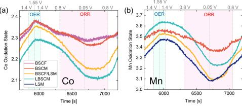
Fig. 5 The operando XAS results of the 5th and 6th CV (zoomed in region from Fig. 4) at the (a) Co and (b) Mn K-edges. The ORR and OER regions are indicated (blue for OER and red for ORR) to highlight the rate of change of oxidation state in these regions.
