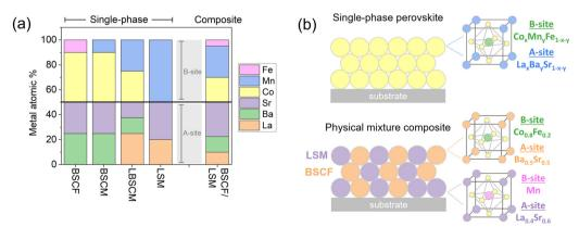
Fig. 1 (a) The metal concentration of the perovskites studied in this work. Oxygen is not included in the percentage. The elements La, Ba, and Sr occupy the A-site of the perovskite structure (ABO<sub>3</sub>) and the elements Co, Mn, and Fe occupy the B-site. (b) Schematic diagram of the catalyst layer for the two design strategies, a single-phase material and a physical mixture composite. The composition is calculated from synthesis stoichiometry
