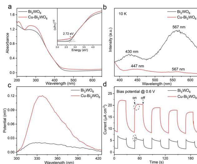
**Fig. 3** (a) UV-vis absorption spectra (Inset: The corresponding Tauc plots), (b) low-temperature (10 K) steady-state photoluminescence emission spectra, (c) SPV spectra and (d) the periodic on/off photocurrent responses of  $\text{Bi}_2\text{WO}_6$  and  $\text{Cu-Bi}_2\text{WO}_6$  samples.
