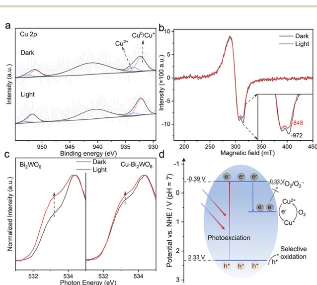
Fig. 4 (a) *In situ* high-resolution Cu 2p XPS spectra and (b) *in situ* ESR spectra of Cu-Bi<sub>2</sub>WO<sub>6</sub> under dark and illumination conditions. (c) *In situ* O K-edge XANES spectra of Bi<sub>2</sub>WO<sub>6</sub> and Cu-Bi<sub>2</sub>WO<sub>6</sub> under dark and illumination conditions. (d) Band structure diagram of Cu-Bi<sub>2</sub>WO<sub>6</sub>.
