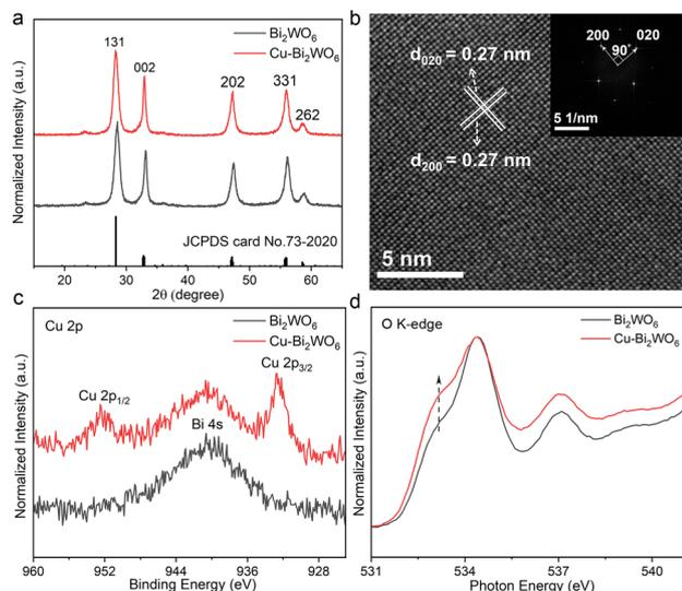
**Fig. 2** (a) XRD patterns of  $\text{Bi}_2\text{WO}_6$  and  $\text{Cu-Bi}_2\text{WO}_6$ . (b) HRTEM image of  $\text{Cu-Bi}_2\text{WO}_6$  (Inset: The corresponding FFT pattern). (c) High-resolution Cu 2p XPS spectra and (d) O K-edge XANES spectra of  $\text{Bi}_2\text{WO}_6$  and  $\text{Cu-Bi}_2\text{WO}_6$ .
