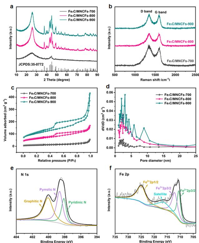
Fig. 2 (a) XRD patterns, (b) Raman spectra, (c) nitrogen adsorption-desorption isotherms, and (d) pore diameter of  $\text{Fe}_3\text{C}/\text{MNCFs}$  with pyrolysis temperatures at 700 °C, 800 °C, and 900 °C. (e) N 1s and (f) Fe 2p spectra of  $\text{Fe}_3\text{C}/\text{MNCFs}-800$ .
