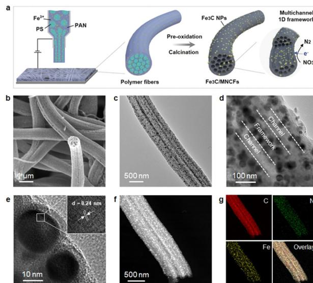
Fig. 1 (a) Illustration for the preparation of  $\text{Fe}_3\text{C}/\text{MNCFs}$ -800 via the electrospinning method and the subsequent pyrolysis. (b) SEM image of  $\text{Fe}_3\text{C}/\text{MNCFs}$ -800. (c) and (d) TEM images of  $\text{Fe}_3\text{C}/\text{MNCFs}$ -800. (e) HR-TEM image of  $\text{Fe}_3\text{C}/\text{MNCFs}$ -800. (f) HAADF-STEM image and (g) elemental mapping of  $\text{Fe}_3\text{C}/\text{MNCFs}$ -800.
