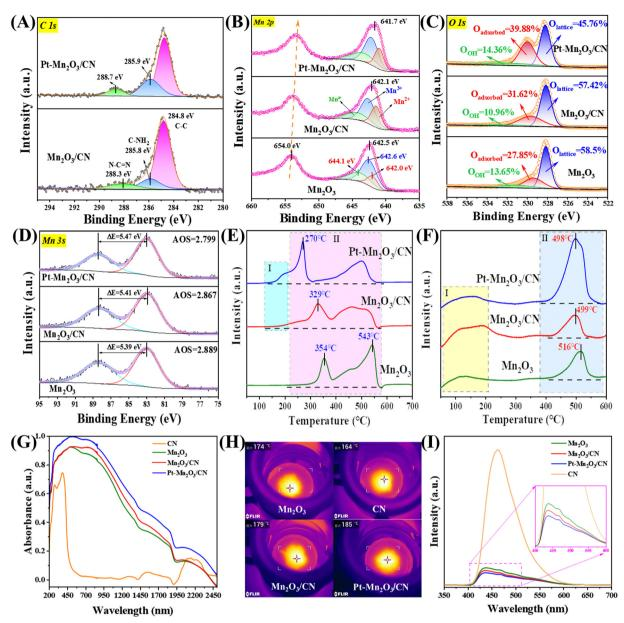
Fig. 4 XPS survey spectra of (A) C 1s, (B) Mn 2p, (C) O 1s, and (D) Mn 3s, (E) H<sub>2</sub>-TPR, (F) O<sub>2</sub>-TPD, (G) UV-Vis-IR absorption spectrum, (H) photothermal conversion temperatures and (I) photoluminescence spectra over different catalysts.
