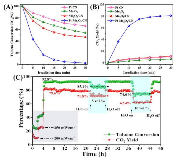
Fig. 3 Photothermal catalytic oxidation of toluene, (A) toluene conversion, and (B) CO<sub>2</sub> yield during the static reaction with 400 ppm toluene over the different catalysts, (C) toluene conversion and CO2 yield during the continuous flow reaction over the Pt-Mn2O3/CN catalysts (full solar spectrum irradiation with 300 mW cm<sup>-2</sup> light intensity, 200 ppm toluene, and WHSV =  $30\,000$  mL g<sup>-1</sup> h<sup>-1</sup>).
