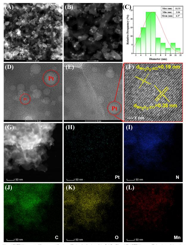
Fig. 2 (A) and (B) TEM images at different magnifications, (C) size distribution of the Pt NPs, (D) and (E) HRTEM images, (F) the shots of the selected area in the panel, (G)–(L) EDS phase mapping of the Pt (blue), O (yellow), Mn (red), N (navy), and C (green), distributions images of the Pt–Mn $_2O_3$ /CN catalyst.
