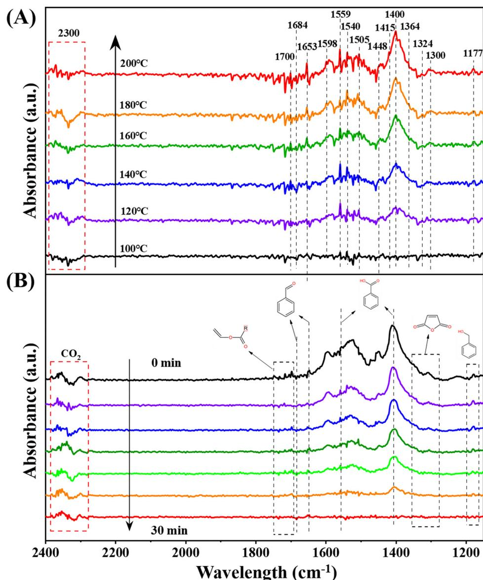
Fig. 5 *In situ* DRIFTS spectra of (A) toluene adsorption at different temperatures and (B) toluene oxidation (1000 ppm toluene +  $\text{O}_2$  +  $\text{N}_2$  feed gas) over Pt- $\text{Mn}_2\text{O}_3/\text{CN}$ .
