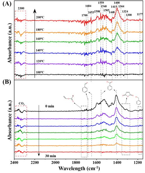
Fig. 5 In situ DRIFTS spectra of (A) toluene adsorption at different temperatures and (B) toluene oxidation (1000 ppm toluene + O<sub>2</sub> + N<sub>2</sub> feed gas) over Pt-Mn<sub>2</sub>O<sub>3</sub>/CN.
